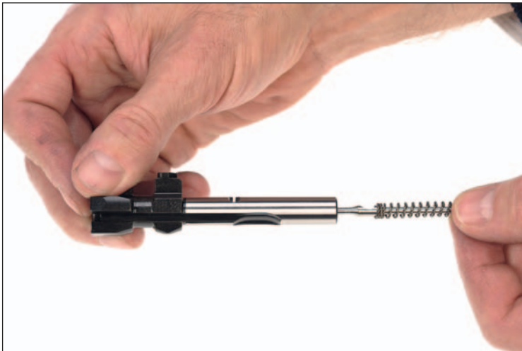
Figure 61: Install firing pin
