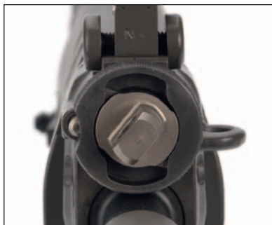
Figure 38: Gas valve in position II
