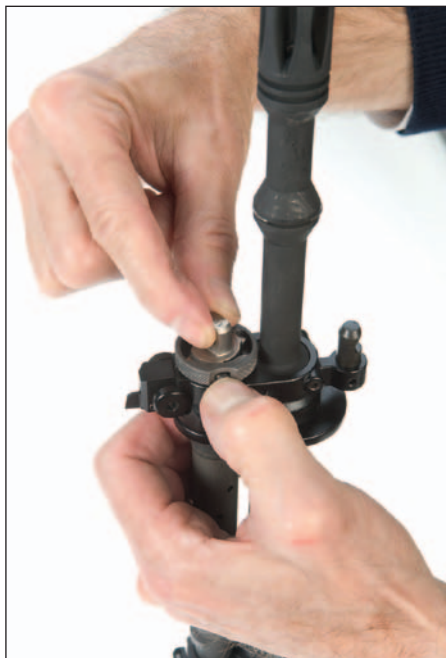
Figure 63: Install gas valve
