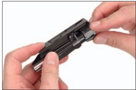
Figure 50: Remove bolt head (rotate)
