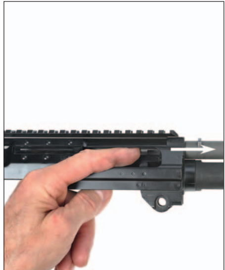
Figure 54: Remove gas piston
