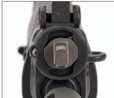
Figure 37: Gas valve in position I
