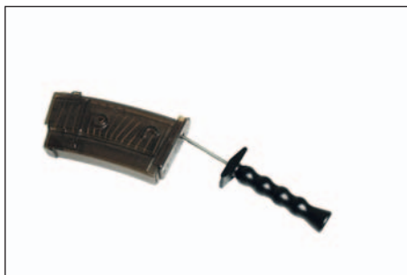
Figure 56: Stripping the magazine
