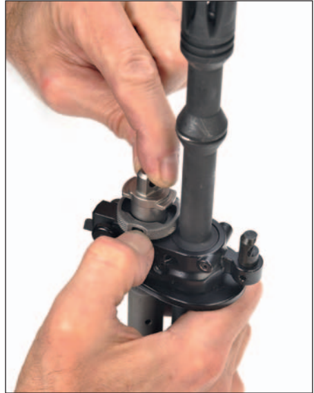
Figure 53: Remove gas valve
