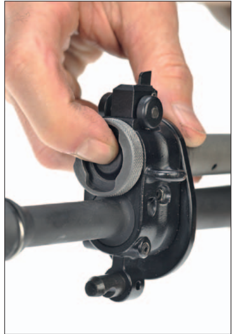
Figure 62: Check gas piston position
