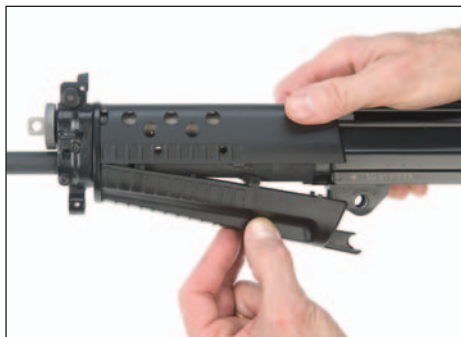
Figure 52: Lift off lower handguard
