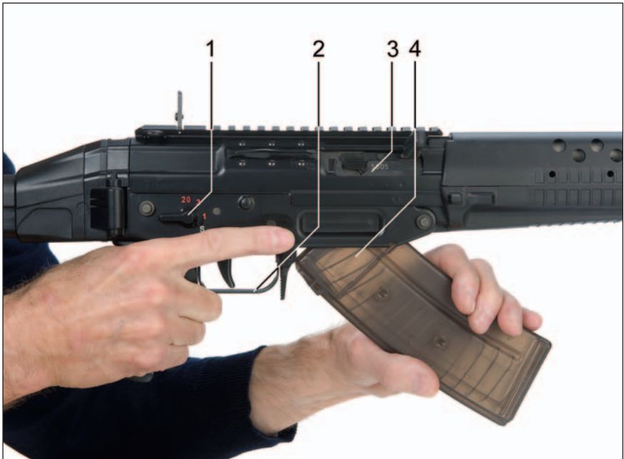
Figure 25: Inserting the magazine
