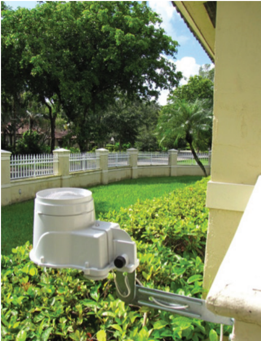
Figure 2. Weather station for evapotranspiration controller for irrigation scheduling (Credits: S. Michael Gutierrez)
