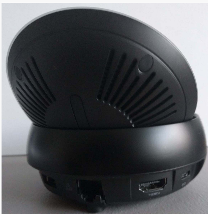
Figure 1131: Samsung DeX, Rear Showing Ports
