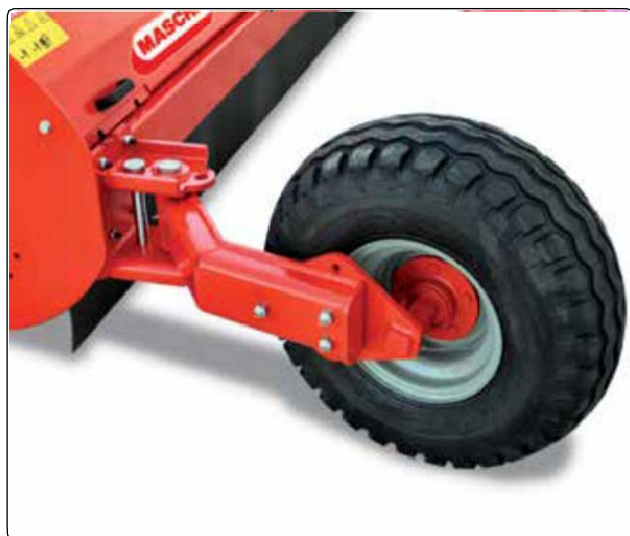
Detail: rear semi-pivoting wheel
