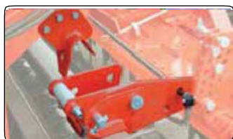
Hopper stands on the roller
