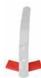
12 in.-wide wings - for shallower working depths
