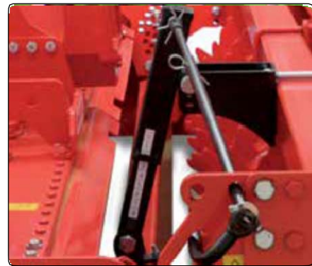
Rear levelling bar with mechanical central adjuster
