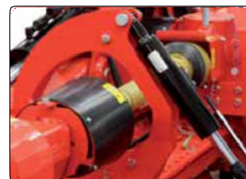
Hydraulic rear roller side adjusters (opt)
