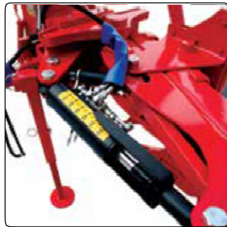
Working width hydraulically variable with parallelogram system (VARIO) on LELIO, SIRO, FURIO
