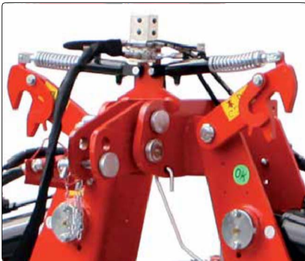
Safety hydraulic locks for transport
