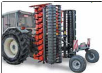
Hydraulically lifted transport trolley
