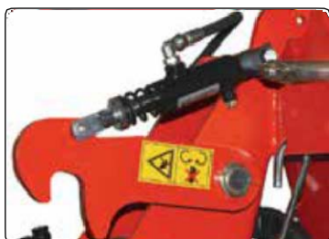
Safety hydraulic locks for transport
