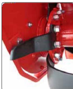
Scraper blade, one for each flank
