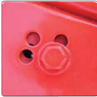
Mechanical adjustable working width by step by step system
