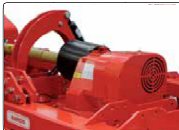
Air cooled side gearboxes
