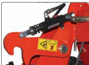
Safety hydraulic locks for transport
