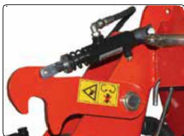
Safety hydraulic locks for transport
