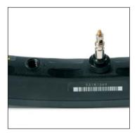
With the valve hole near you, place the rim such that the raised indicator bump is to the left of the valve hole.
