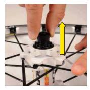
Remove the disc side frame support by pulling on it.
