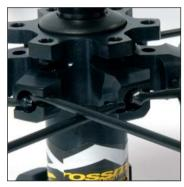
Insert the heads of these spokes into the hub slots on the disc side: the nonbraking spokes into the inside notches, the braking spokes into the outside notches.
