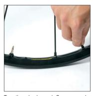
Turn the wheel round. Screw a spoke 2 turns into the third hole to the right of the valve hole. Do likewise for all the non-braking spokes, 1 hole in 4 on the rim.
