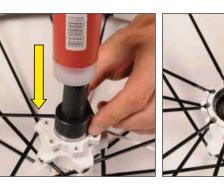
Position the drive side bearing with the disc side bearing seal. Refit the bearing with press kit M40119.
