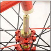
Fit the new bearings with press kit 996 887 01.
