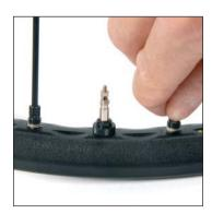
And finally, screw a spoke 2 turns into the first hole to the right of the valve hole. Do likewise for all the braking spokes, 1 hole in 4 on the rim.
