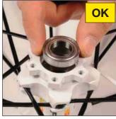
In order to ensure a perfect seal of the free wheel mechanism, the bearings of the hub body must be mounted with the disc side seal.
