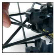
Insert the heads of these spokes into the hub slots on the non-disc side: the non-braking spokes into the inside notches, the braking spokes into the outside notches.
