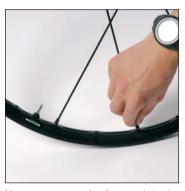
Now screw a spoke 2 turns into the third hole to the right of the valve hole. Do likewise for all the braking spokes, 1 hole in 4 on the rim.
