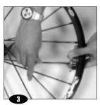
CAUTION : manipulating the integrated nipples greatly affects the spoke tension and consequently the wheel adjustment.
