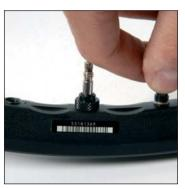
Screw a spoke 2 turns into the first hole to the right of the valve hole. Do likewise for all the non-braking spokes, 1 hole in 4 on the rim.
