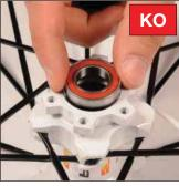
Fit the new non-drive side bearing with press kit M40119.
