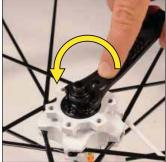
Completely unscrew the adjustment nut with the hub wrench 325 423 01.
