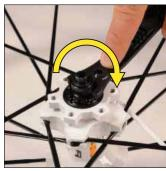
Refit the adjustment nut and the frame support.
