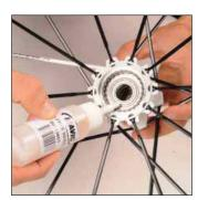
Clean the hub body and fill three ratchet teeth with oil 996 136 01 and refit the axle and free wheel mechanism assembly.
