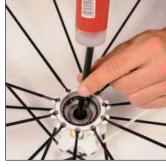
Using the press kit, remove the two bearings from the inside. Clean with a dry cloth if necessary.
