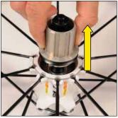
You can now remove the axle and free wheel mechanism assembly.
