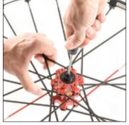
To unclip them, push them in turn via the inside of the hub using a quickrelease rod.
