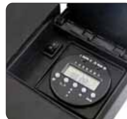
Figure 19: Positioning the lighting control panel
