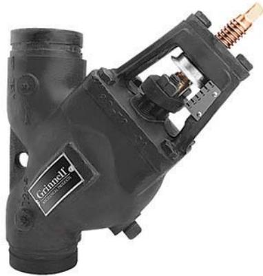
The GRINNELL Model TD830 Triple Duty Valve is designed for installation in pump discharge piping where it functions as a spring-loaded silent check valve, a balancing valve, and a shut-off valve.
