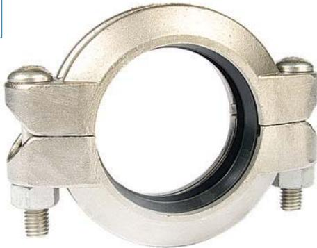
The GRINNELL Figure 472 Rigid Coupling is made of cast 316L stainless steel and is capable of pressure up to 600 psi (41,4 bar).
