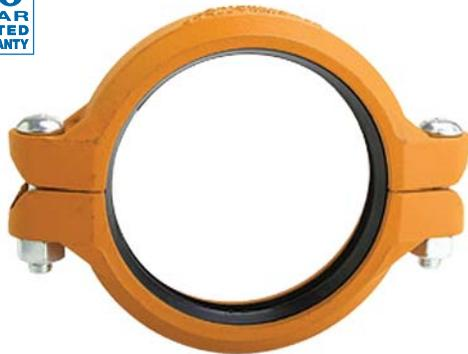
The GRINNELL Figure 705 Flexible Coupling allows for angular and linear deflection, thermal expansion and contraction, and misalignments of pipe. It is capable of pressures up to 500 psi (34,5 bar), depending on pipe size and wall thickness. Suitable for use in a variety of applications, the GRINNELL Figure 705 Coupling provides a dependable method of joining pipe.
