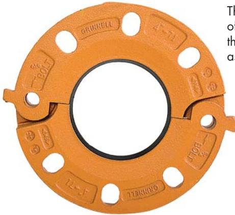
The Figure 71 Flange Adapter is capable of pressures up to 300 psi (20,7 bar) depending on pipe size and wall thickness. It provides a direct transition from flanged components to a grooved piping system. I.P.S. size flange bolt patterns conform to PN10/PN16
