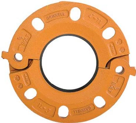
The Figure 71 Flange Adapter is capable of pressures up to 300 psi (20,7 bar) depending on pipe size and wall thickness. It provides a direct transition from flanged components to a grooved piping system. I.P.S. size flange bolt patterns conform to AS2129 Table E.
