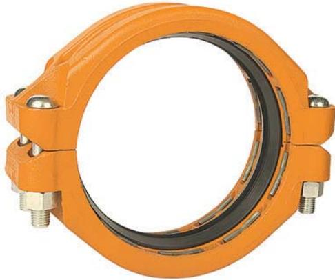
The GRINNELL Figure 909 Plain End Coupling utilizes hardened gripping teeth to securely grip onto plain and beveled end pipe surfaces. It is capable of pressures up to 750 psi (51,7 bar) depending on pipe size and wall thickness.
