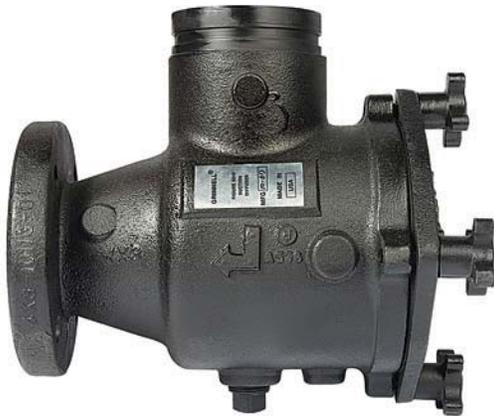
The GRINNELL Figure S810 Suction Diffuser is compact and rugged for direct mounting to the suction side of a pump in either a horizontal or vertical position. In addition to removing foreign particles, this diffuser also provides proper flow conditions to the pump. Where space is limited, this diffuser can be used to replace the straight pipe normally required to reduce turbulence.
