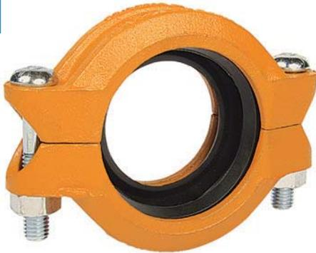
The GRINNELL Figure 716 Flexible Reducing Coupling allows for a direct transition between two different pipe sizes and replaces two couplings and a reducing fitting. It is capable of pressures up to 500 psi (34,5 bar) depending on pipe size and wall thickness. A flexible reducing coupling is not recommended for low-temperature applications.
