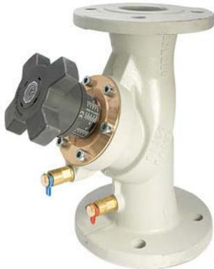
The GRINNELL Model CB800 Balancing Valve provides features for achieving accurate and efficient balancing of hydronic heating or cooling systems. One valve serves five functions: throttling, measuring (pressure and temperature), positive shutoff, draining, and filling. The GRINNELL Flange-by-Flange Model CB800 Valve, available in sizes 2½" to 12" (65mm to 300mm), is composed of cast iron.
