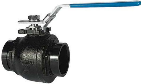
GRINNELL Model BV835 Ball Valves provide for efficient control of fluid in piping systems. Flow may be from either direction, and the valves may be positioned in any orientation. The valves are furnished with grooved ends for use with GRINNELL Grooved Couplings. The handle is provided with a device for padlocking in either the open or closed position.
