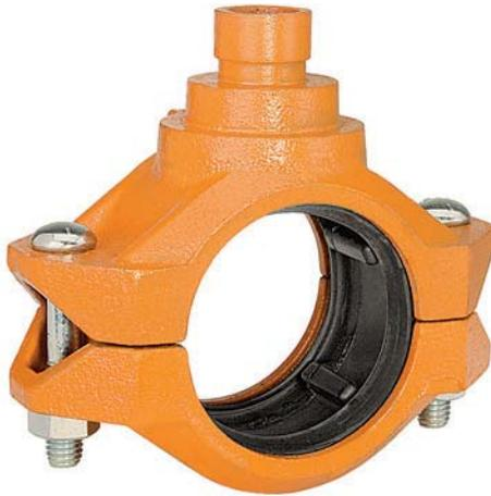
The GRINNELL Figure 702 Mechanical Outlet Coupling has the combined features of a coupling and a reducing outlet, eliminating the need for a mechanical tee or other associated couplings. The coupling is available in grooved, male-threaded, or female-threaded outlets. This design makes installation faster, safer, and more cost effective on the job site.
