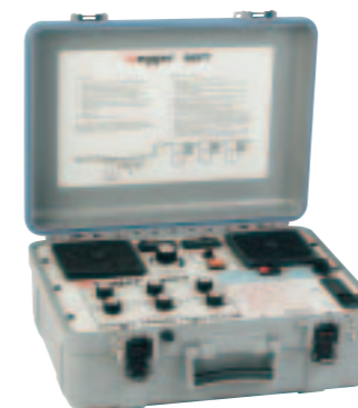
The Battery Ground-Fault Tracer is an economical, manually-balanced instrument that identifies, tracks and locates ground faults in ungrounded d.c. battery systems - on-line. It is particularly effective in a high electrical noise environments, as the strength of the test current can be adjusted
