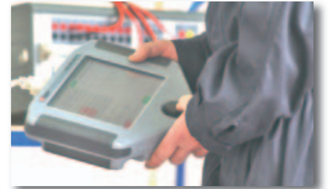
MPRT relay test set with touch view interface makes it easy to perform manual and semi-automatic relay testing
