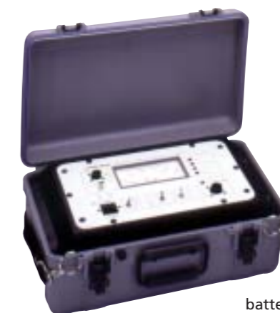
BGL simplifies fault tracing by identifying fault characteristic (resistive and capacitive) magnitudes
