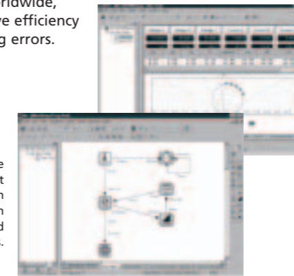
AVTS can display the voltage and current output waveforms in time sequence with the binary inputs and outputs.
