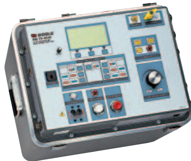
Delta 2000 is ideal for tan delta testing on transformers
