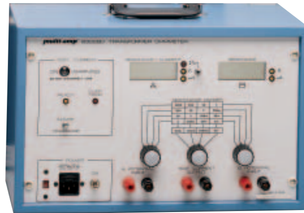
A lightweight, field portable unit that safely and accurately measures the DC winding resistance of all types of transformers and rotating machines
