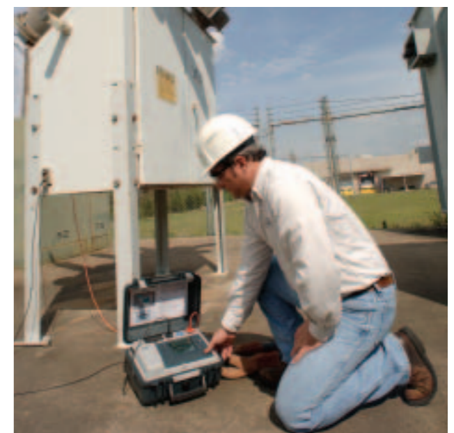
CATIV protection gives confidence when insulation testing outside
