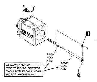
FIGURE 4-23. TACH RETAINING SCREW AND CLIP
