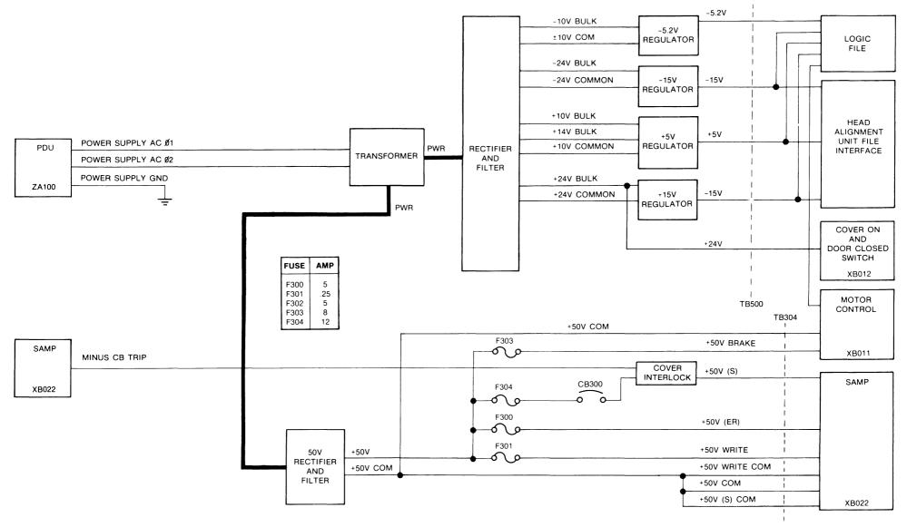
FIGURE 3-80. DC BULK VOLTAGES, VOLTAGE REGULATORS, AND SERVO VOLTAGES
