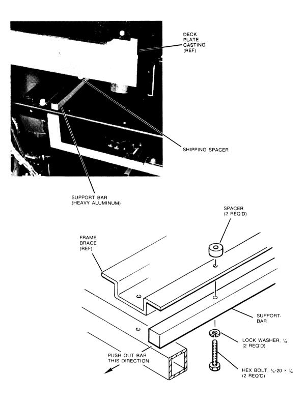
FIGURE 2-5. SHIPPING SPACERS AND SUPPORT BAR
