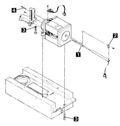
FIGURE 4-17. ACTUATOR MECHANISM
