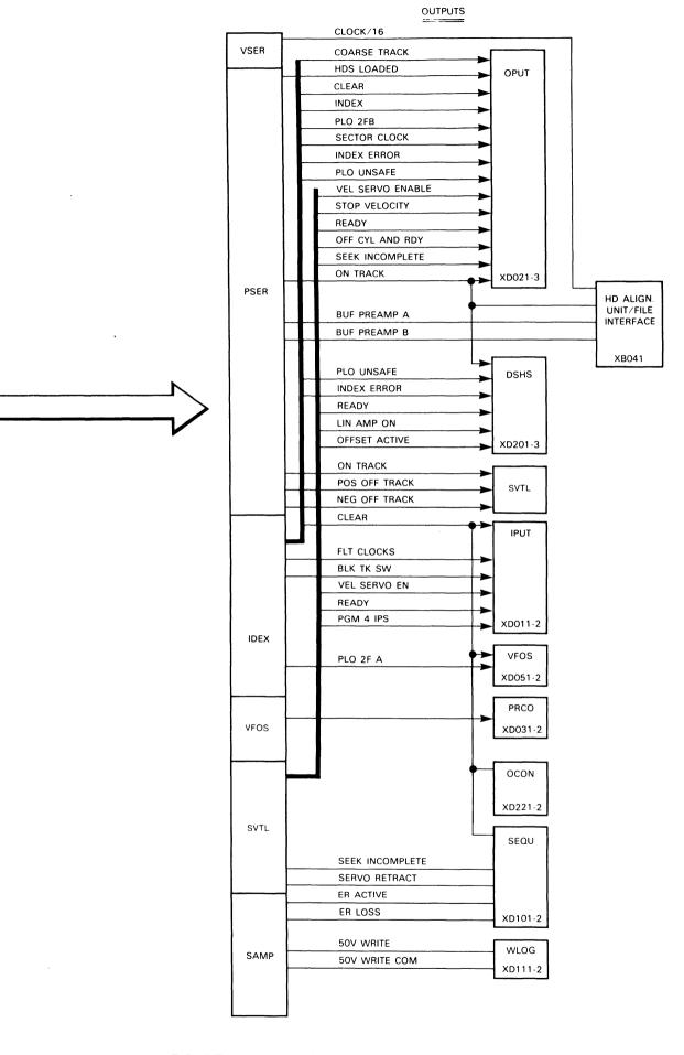
FIGURE 3-32. SERVO SYSTEM INPUTS AND OUTPUTS (Part 2 of 2)
