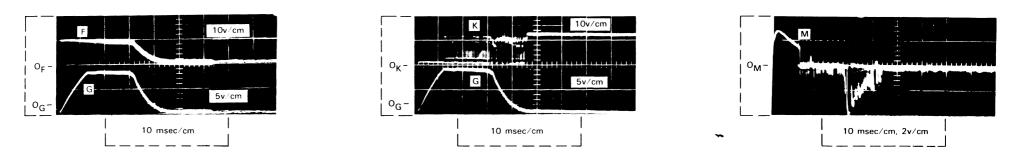
FIGURE 3-58. SERVO SYSTEM WAVEFORMS (Part 6 of 6) - FOUR HUNDRED TRACK SEEK FORWARD
