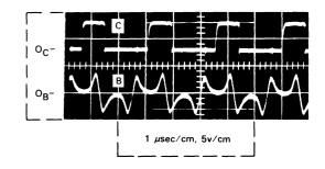
"B" and "E" are shown below for the Head Offtrack (away from spindle) condition.
