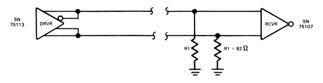
(b) Unidirectional Driver/Receiver Configuration
