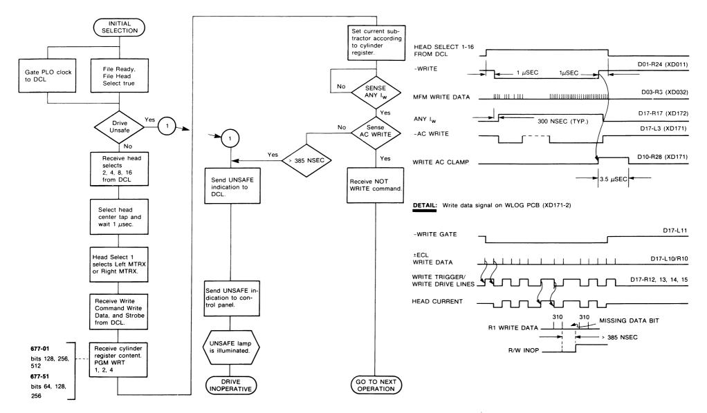
FIGURE 3-73 WRITE OPERATION FLOWCHART AND TIMING
