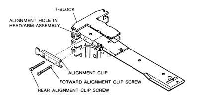
FIGURE 4-5. HEAD ALIGNMENT CLIP AND SCREWS
