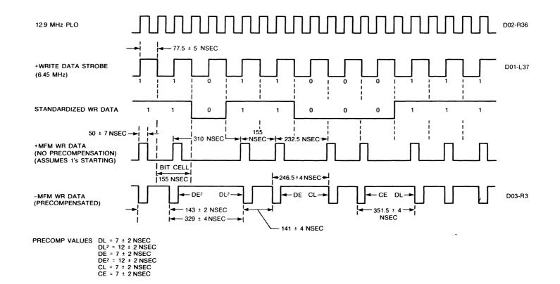
FIGURE 3-4. WRITE DATA TIMING
