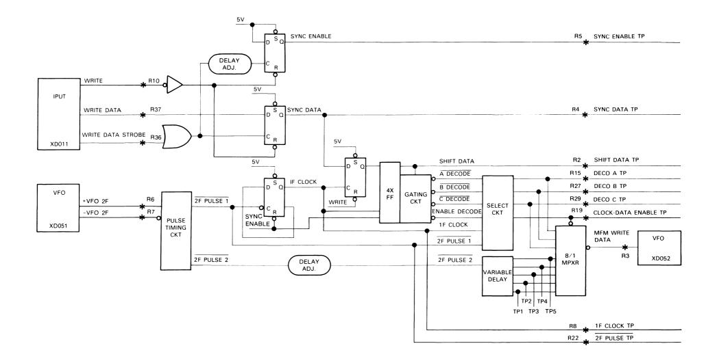
FIGURE 3-7. PRECOMPENSATION PCB (PRCO PCB, D03 LOCATION)
