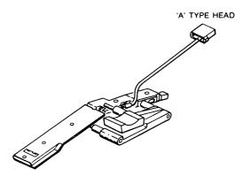
FIGURE 4-7. HEAD INSTALLATION TOOL IN 'A' TYPE HEAD
