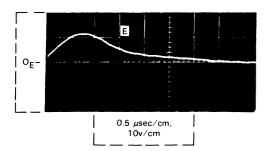
"H" shown below is the velocity error (D14 R11). It is the output of the Velocity Error Amp which reflects the difference between actual velocity (tach) and desired velocity (curve). "J" is UNGATED ACCELERATE FWD (D14 R14). It is generated by comparing Velocity Error to 25 KHz sawtooth.
