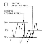
FIGURE 3-29. CARRIER SIGNAL FROM CENTERED SERVO HEAD
