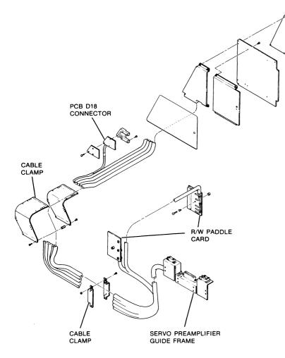
10. Remove screws from servo preamplifier guide frame, which holds bracket containing servo preamplifier connector, and jacks disconnected in preceding step 9.
