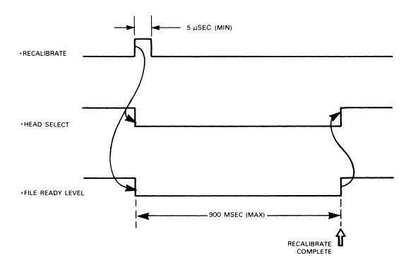
FIGURE 1-14. RECALIBRATE TIMING
