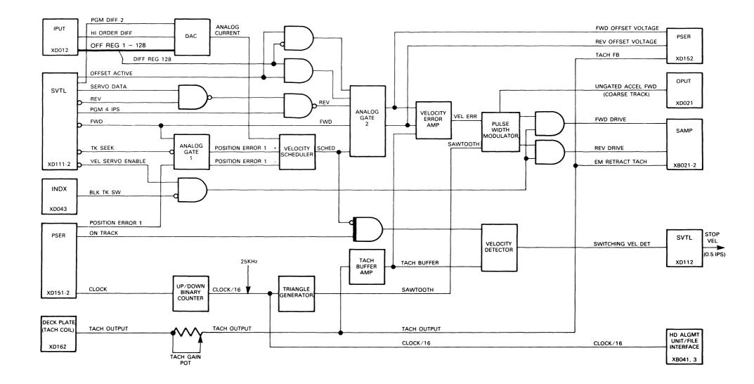
FIGURE 3-42. VELOCITY SERVO PCB
