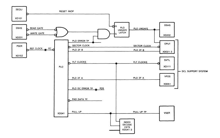
FIGURE 3-16. PLO INPUTS AND OUTPUTS
