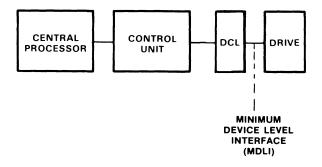
As indicated above, a drive transfers data to the system through the MDLI to its attached DCL.
