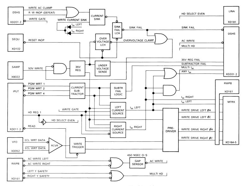
FIGURE 3-72. WRITE LOGIC PCB
