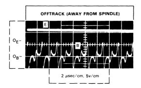
"D" shown below is GATE NEGATIVE (D15 R35). It gates second-negative peaks into the Negative Peak Detector. As previously identified, "B" is the Carrier Amp output.
