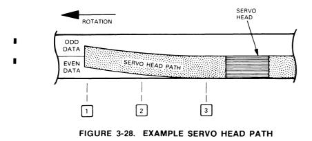
At point 1 in the head path shown above, the servo head is centered over the border between even and odd data. The E and O signals (at the output of the servo preamp), in terms of percent of maximum signal amplitude, are shown in the illustration below.
