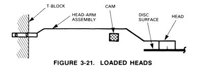
**Retract.** To perform a retract operation, heads are unloaded and then retracted from the pack. The sketch below shows orientation of mechanical components when heads are unloaded. As shown, the bend in any head-arm assembly is contacting a cam surface when heads are unloaded.
