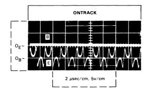
"C" shown below is GATE POSITIVE (D15 R33). It gates the second-positive peaks into the Positive Peak Detector. As previously identified, "B" is the Carrier Amp output.
