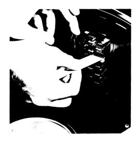
FIGURE 4-3. CLEANING HEADS IN DRIVE
