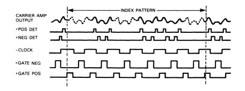
FIGURE 3-45. SERVO CLOCKING FOR INDEX
