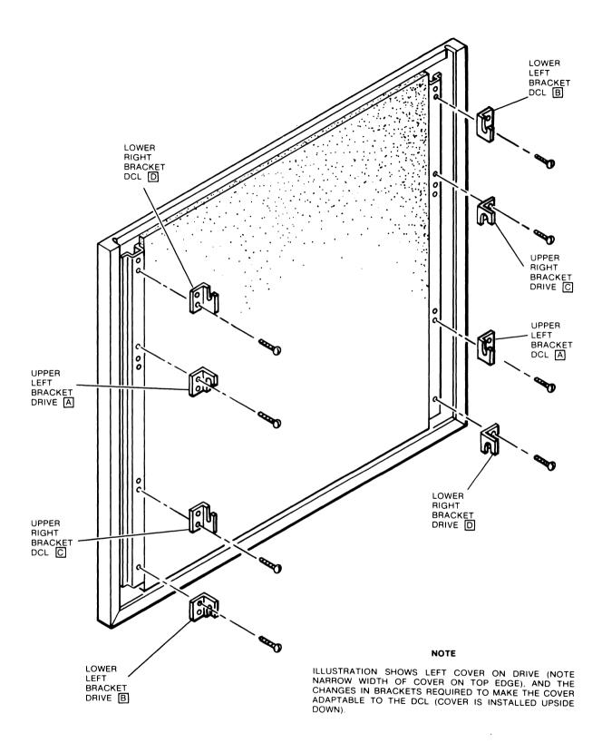
FIGURE 2-9. CONVERTING DRIVE COVER TO DCL COVER
