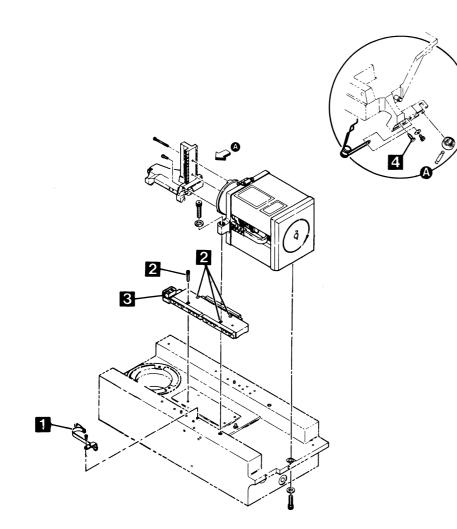
FIGURE 4-19. CARRIAGE T-BLOCK ASSEMBLY AND WAY
