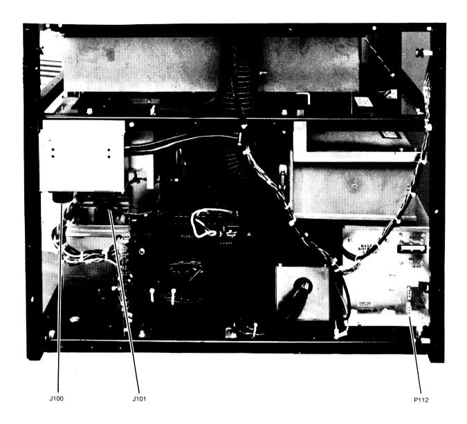
FIGURE 1-21. EXTERNAL CABLE CONNECTORS
