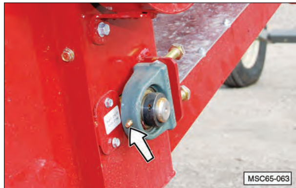
Conveyor Belt Upper Roller
