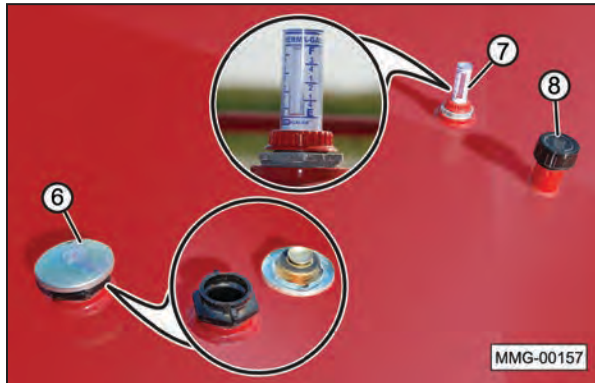
(6) Fuel tank fill opening with vented and lockable cap. (7) Fill level indicator. (8) Tank vent.
