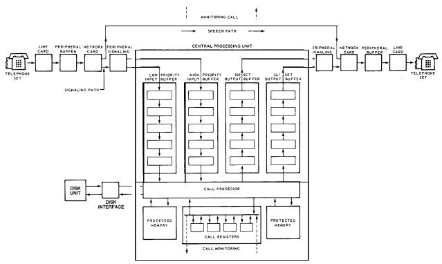
NOTE: BUFFERS AND REGISTERS ARE CONTAINED IN THE UNPROTECTED DATA STORE
