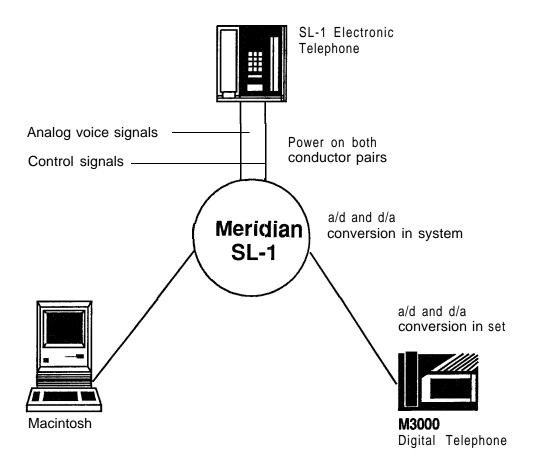
The Meridian SL-1 architecture uses a star technique that permits uniform distributed wiring methods to connect each peripheral device to the switching system. This approach provides significant benefits in the area of administration, installation, maintenance and reliability.
