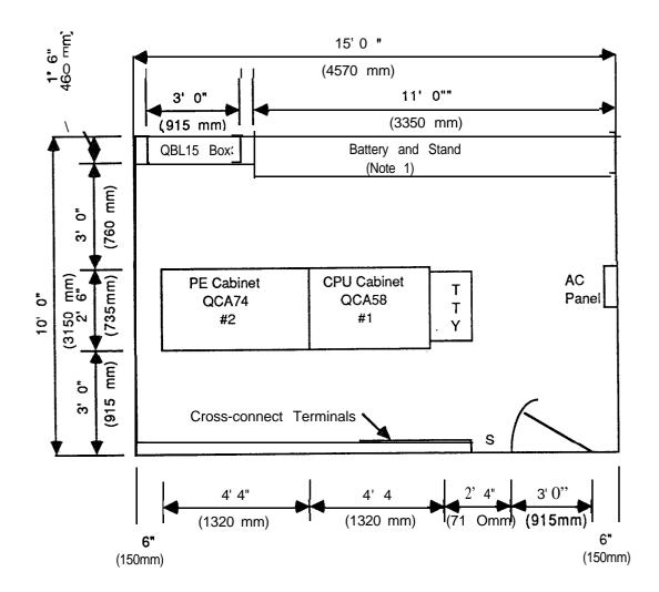
FIGURE 6- 1: TYPICAL MERIDIAN SL- 1NT FLOOR PLAN
