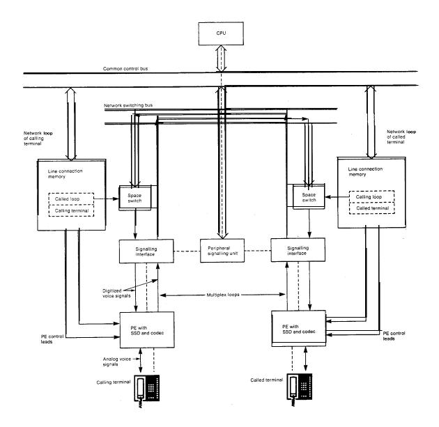
This illustration shows how a call is set up on the Meridian SL-1. When a user lifts the handset to make a call, an SSD in the PE detects a change of state in the terminal. Under control of the peripheral signaling device, a message is sent to the CPU indicating that
