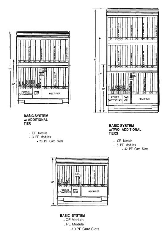
FIGURE 5-45: MERIDIAN SL-1ST INITIAL CABINET CONFIGURATIONS
