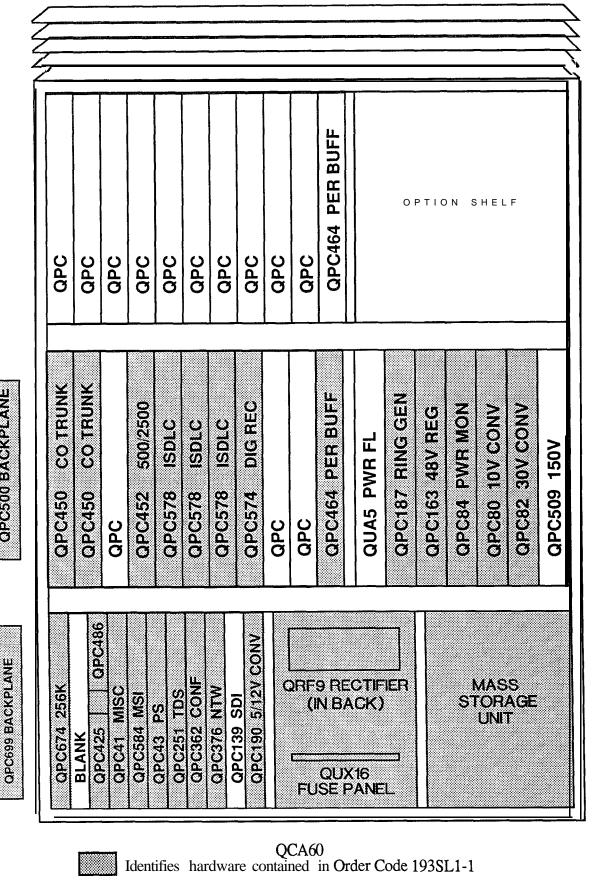
FIGURE 10-2: MERIDIAN SL-1S PRE-PACKAGED SYSTEM (32 LINE/8 TRUNK)
