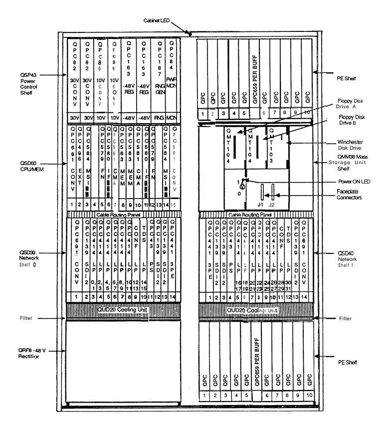
FIGURE 5-34: MERIDIAN SL-1NT QCA58 CABINET - FRONT VIEW
