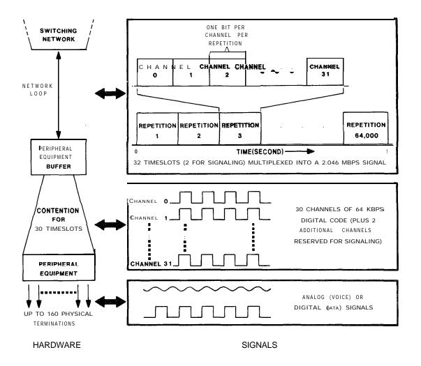
This figure illustrates the principle of time division multiplexing as used in the multiplexed loops. Thirty-two digital signals are sent over a common path by transmitting them sequentially at different instants of time. As a result of eight-bit PCM encoding, the individual signals are at 64 kilobits per second, giving a combined rate of 2.048 megabits per second for each loop. This may be thought of as 64,000 repetitions per second of a sequence of 32 time slots or channels.
