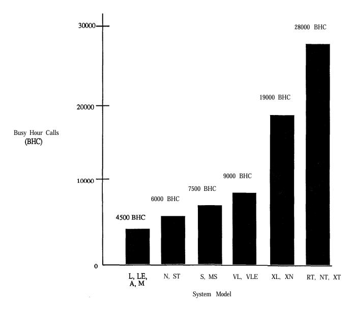
FIGURE 9-1: MERIDIAN SL-1 CALL HANDLING CAPACITY
