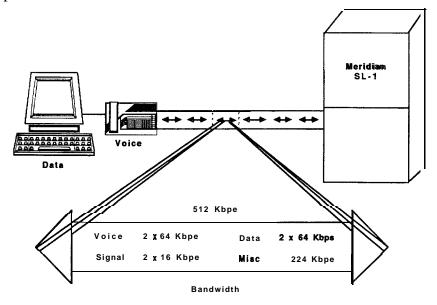
FIGURE 3-13: TIME COMPRESSION MULTIPLEXING
