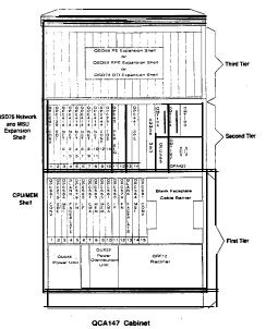
FIGURE 5-3: MERIDIAN SL- 1**ST** EQUIPMENTCABINET
