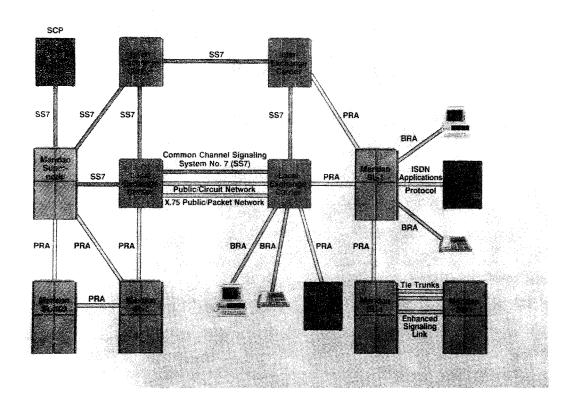
Meridian Customer Defined Networking is the basis for custom private and hybrid networks that use a mix of *ISDN* interfaces, enhanced *SS7* signaling, circuit and packet switching, bandwidth management, and advanced networking applications.
