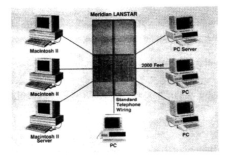
The Meridian LANSTAR is a star configuration providing greater security and reliability than other network designs. The Meridian LANSTAR packet transport's 40 Mbps bandwidth combined with 2.56 Mbps full duplex dedicated to each personal computer provides superior performance and throughput to networked personal computers.
