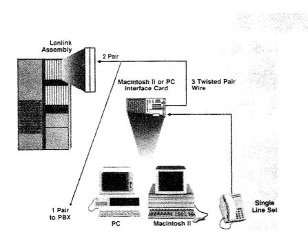
A LANSTAR PC or Macintosh II Interface Card is installed in each personal computer. A second RJ-11 jack is provided on the card to plug in a telephone. Standard telephone wiring connects the personal computer to the LANLINK Assembly residing in the Meridian LANSTAR packet transport.
