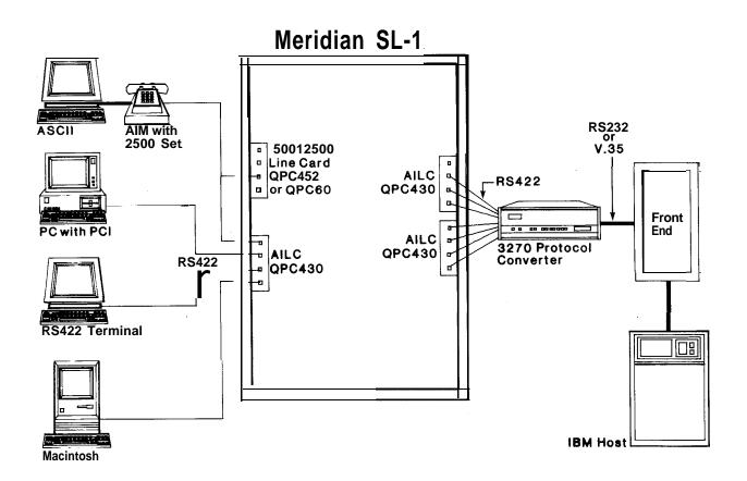
FIGURE 8-33: ASYNCHRONOUS INTERFACE LINE CARD
