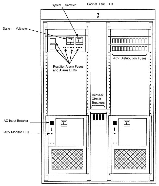
FIGURE 5-6: MERIDIAN SL-1XN/XT CENTRALIZED POWER CABINET
