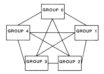
In the multi-group arrangement, junctors provide an additional switching stage to extend the originating and terminating network loops from any one group to any other. Five network groups may be interconnected to constitute the capacity of the digital switching matrix.
