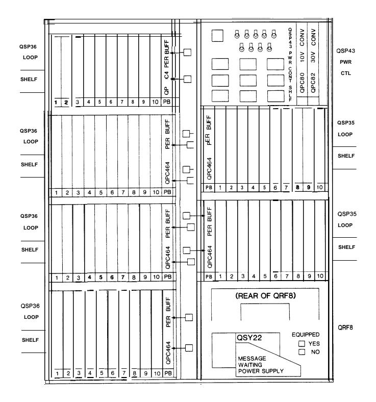
FIGURE 5-21: MERIDIAN SL-1N QCA58 CABINET - REAR VIEW
