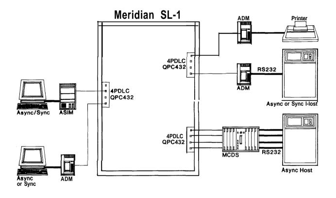
FIGURE 8-32: FOUR PORT DATA LINE CARD
