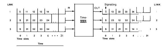
With time-space switching, a conversation occupying any time slot on any inlet link can be switched to any time slot on any outlet link. For example, the conversation in time slot 1 on link 1 (denoted by 11) is switched to slot 3 on link 3. However, a conversation need not necessarily encounter any change in space or time position (eg. conversation 24).
