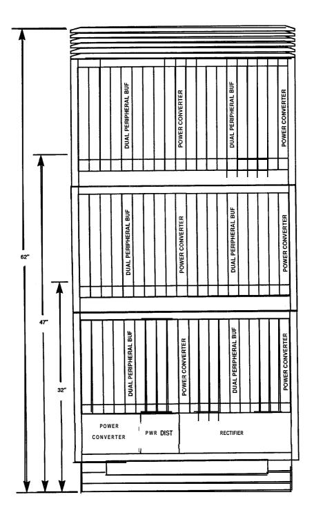
FIGURE 5-48: MERIDIAN SL-1ST/RT PE EXPANSION CABINET
