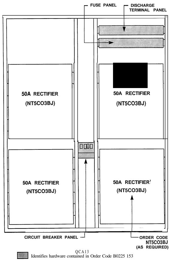
FIGURE 10-21: MERIDIAN **SL-1XT** SUPPLEMENTARY POWER CABINET ASSEMBLY
