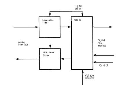
FIGURE 3-3: SINGLE CHANNEL CODEC
