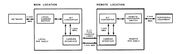
FIGURE 3-5: REMOTE PERIPHERAL EQUIPMENT
