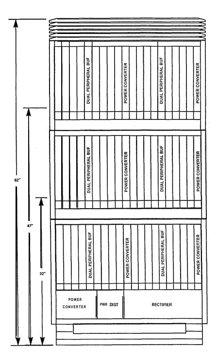
FIGURE 5-A5: MERIDIAN SL-1 ST/RT PE EXPANSION CABINET
