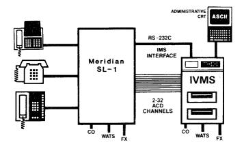
The Integrated Voice Messaging System (*IVMS*) illustrates once again the versatility of the Meridian SL-1. An *auxiliary* processor interacts with the latter to provide sophisticated voice messaging capabilities to the user.
