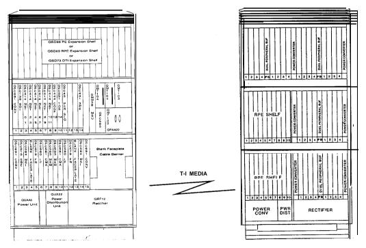
FIGURE 5-A4: MERIDIAN SL-1ST/RT - TYPICAL RPE CONFIGURATION
