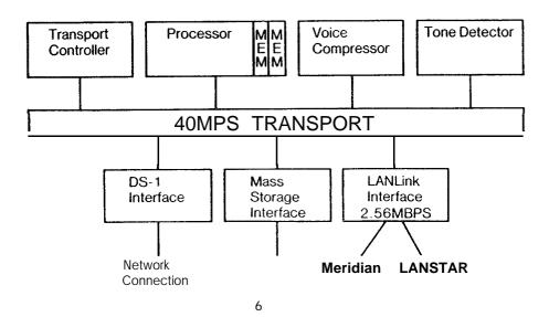
FIGURE 3-29: PACKET TRANSPORT ELEMENTS
