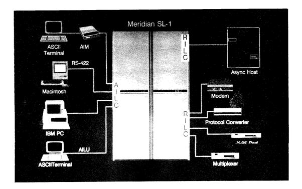
FIGURE S-34: RS-232C INTERFACE LINE CARD
