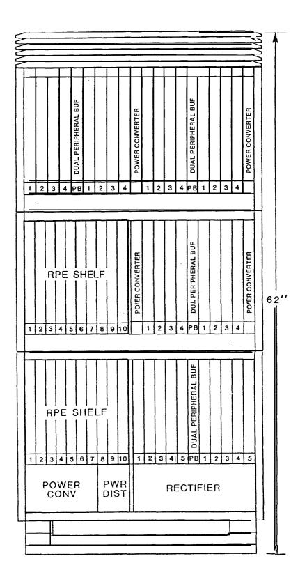
FIGURE 5-54: MERIDIAN SL-1 RPE CABINET CONFIGURATION
