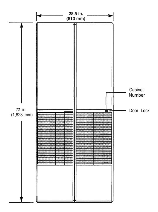
FIGURE 5-4: MERIDIAN SL-1 PACKET TRANSPORT CABINET
