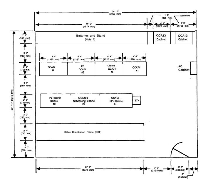
FIGURE 6-2: TYPICAL MERIDIAN SL-1XT FLOOR PLAN
