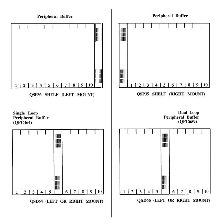
FIGURE 5-50: PERIPHERAL EQUIPMENT SHELF ARRANGEMENTS
