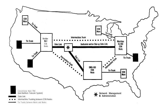
ESN provides a custom designed network *configuration* capable of supporting voice and data communications over a widely dispersed national network with numerous locations.
