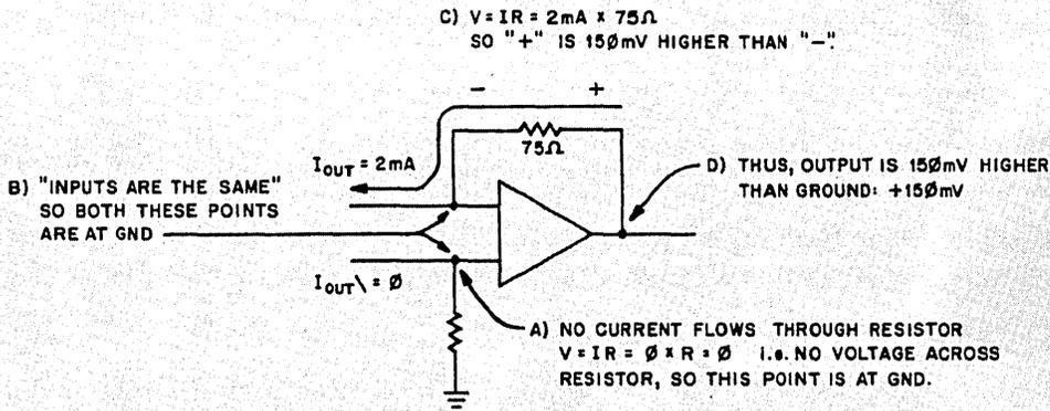
Figure 3C - Outputting A Byte Of "Zeros"
