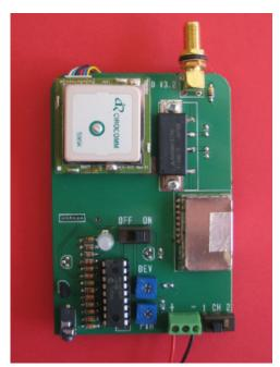
The selector switch, located near the center of the PC board, is a two position switch. Even when left off, the batteries should be removed for extended storage to prevent leakage and damage to the device.
