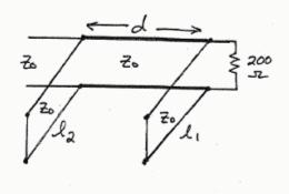
Plots of return loss vs. f/f for these six solutions are shown on the following page. (only 4 curves could be plotted per graph). These results show that the tuner of solution (b-1), the series stub tuner, gives the best bandwidth. This is probably because the stub length and line length are shortest for this cash, giving the smallest frequency variation.
