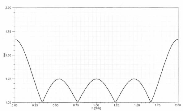
5.20 From (5.61) and (5.60b),  $\Gamma(\theta) = A e^{-2j\theta} T_2 (\text{alc } \theta \text{m } \cos \theta) = A e^{-2j\theta} \left[ \text{alc}^2 \theta \text{m } (1 + \cos 2\theta) - 1 \right]$   $\Gamma(0) = A T_2 (\text{alc } \theta \text{m}) = \left| \frac{Z_L - Z_0}{Z_J + Z_0} \right| = \frac{R - 1}{R + 1} = 0.2 \quad ; \quad A = \Gamma \text{m} = 0.05$
