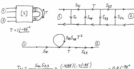
$$T_{21} = \frac{S_{41}S_{23}}{1 - S_{33}S_{44}T^2} = \frac{(.4/45)(.7/-45)}{1 - (.6/45)(.5/45)(1/-90)} = 0.4/-90^{\circ}$$
