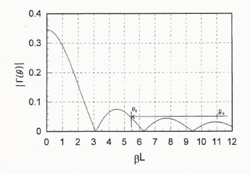
We see that the lower frequency limit for  $|\Gamma| \leq 0.05$  is  $\theta_1 = 5.5$ . To obtain 100% bandwidth, we must have,
