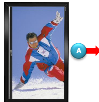
Channel D video output on vertically-oriented widescreen monitor with Output Rotation = Clockwise & Pan Control RIGHT
