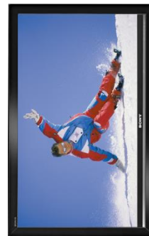
Channel D video output on vertically-oriented widescreen monitor with Output Rotation = None
