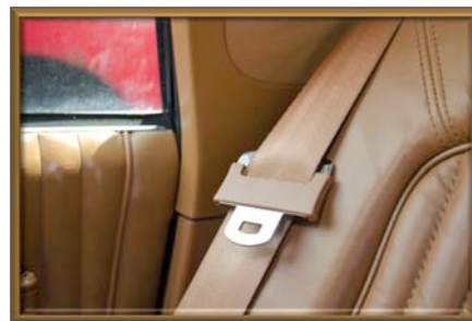
Locking latchplate with plastic piece
