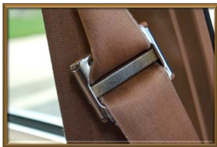
Locking latchplate with sliding metal piece – front and back
