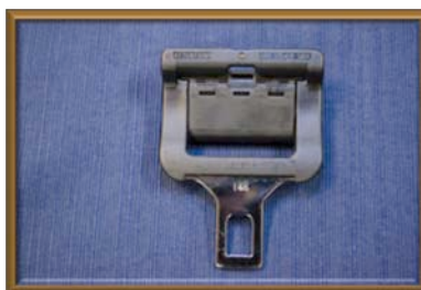
Locking parts from a switchable latchplate – front and back
