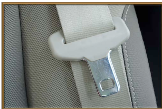
Sliding latchplate found only on lap-and-shoulder systems
