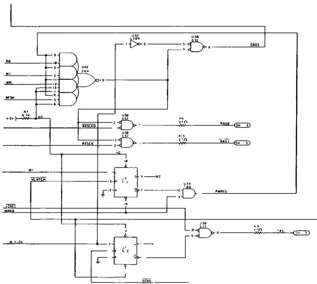
Figure 2-9. Video RAM and DRAM Timing Circuit.
