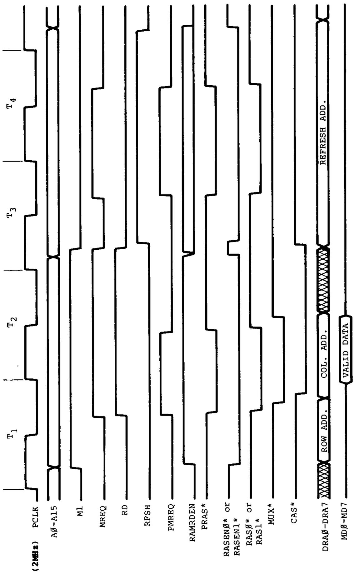
Figure 3-8. M1 Cycle Timing (2MHz) 100ns/dir.
