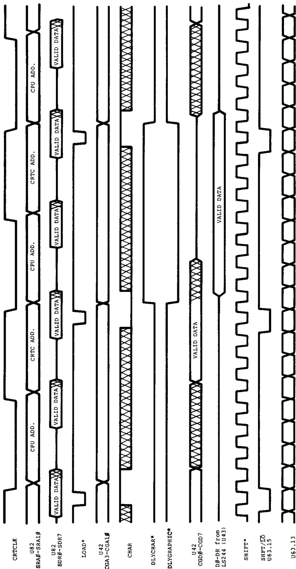
Figure 3-13. Video Circuit Timing
