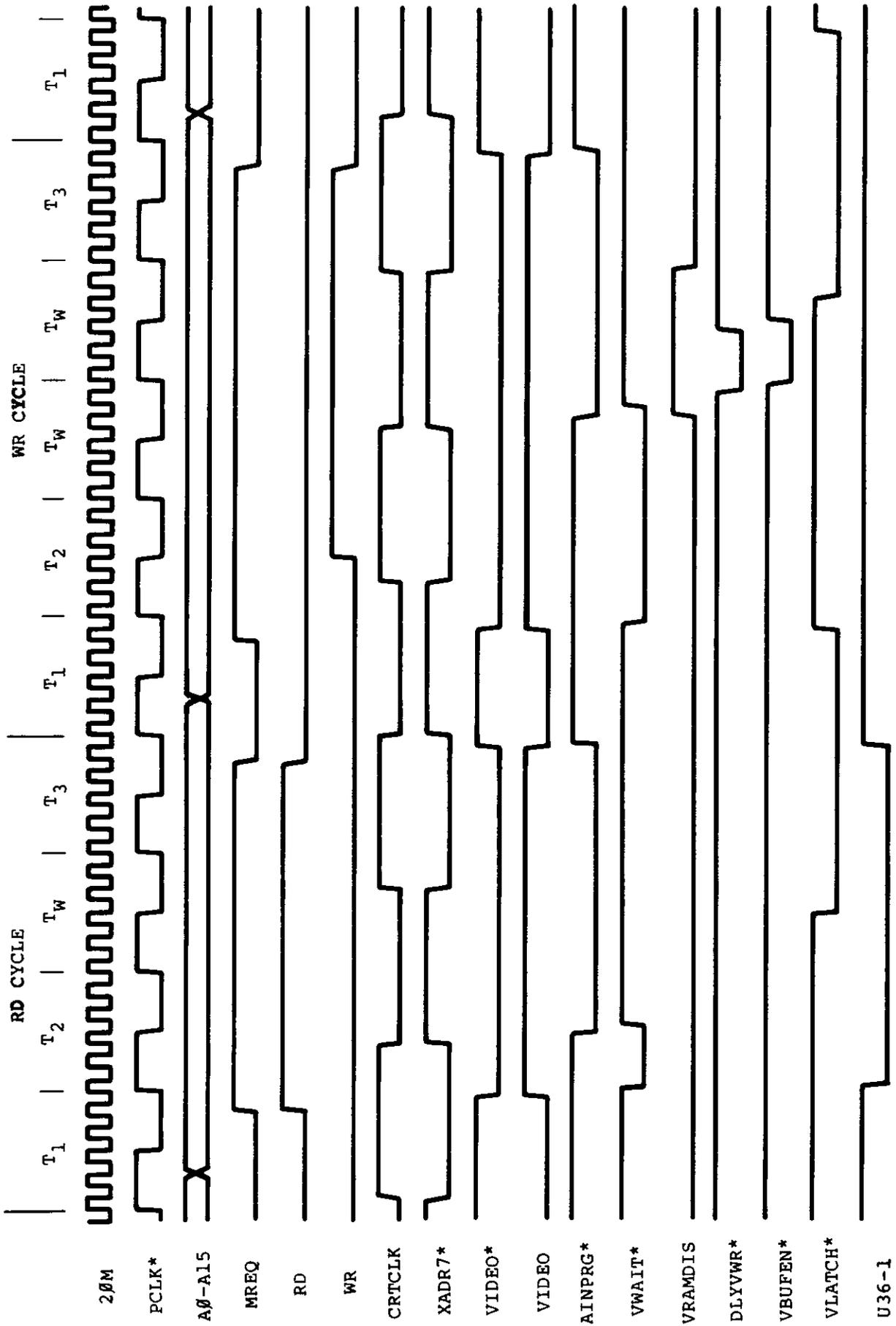
Figure 2-8. Video RAM CPU Access Timing
