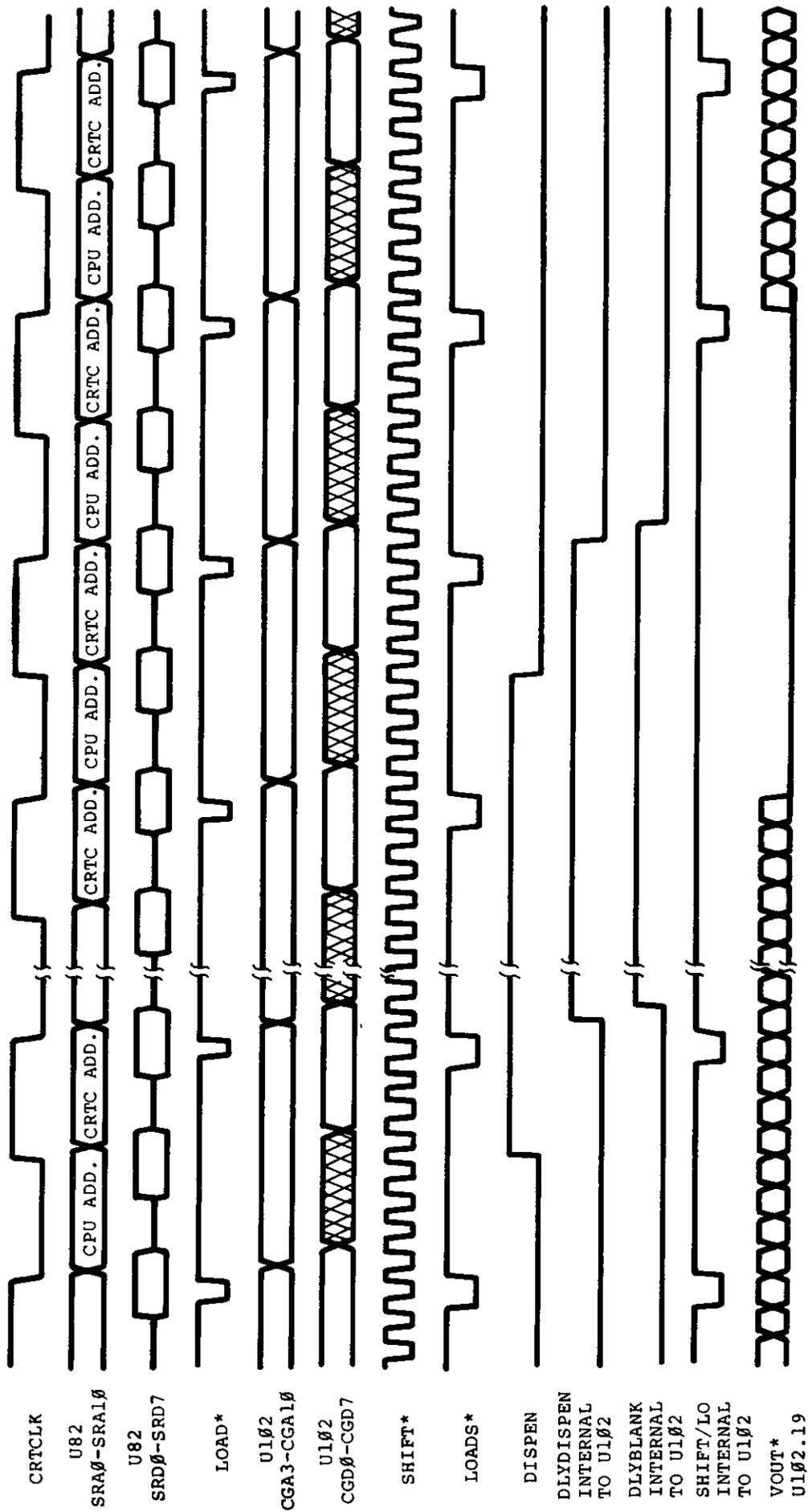
Figure 4-13. Video Blanking Timing
