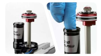
Use a pick to remove the retention clip from the IFP reservoir.
