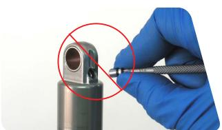
Remove and replace the top out bumper on the damper body.
