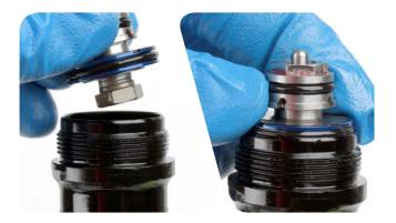
Thread the IFP reservoir onto the eyelet by hand. Use a torque wrench with 27 mm crowfoot to tighten the IFP reservoir to 8.4 N·m (75 in-lb).
