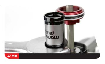
**Monarch Plus™ RC3 Only:** Use your fingers to remove the compression assembly from the IFP reservoir or eyelet.
