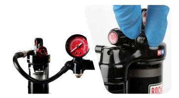
**DebonAir**<sup>™</sup> **Air Cans only:** Use a shock pump to pressurize the shock to the desired air pressure. After adding air to the shock, the pressure will need to be equalized between the shock chambers.
