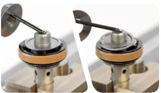
Apply 242® Blue Loctite® only on the threads of the nut, then Apply 242\* Blue Loctile only on the timedas 5. thread the nut onto the damper shaft. Use a torque wrench with a 12 mm socket to tighten the main piston nut to 4.5 N m (40 in-lb).
