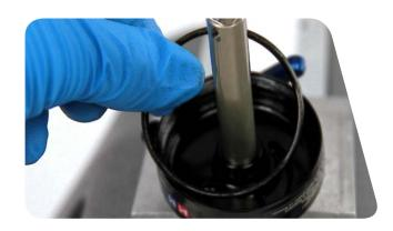
Install the seal head/air piston onto the damper shaft.
