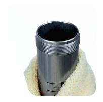
Pour new RockShox 3wt suspension fluid into the damper body until it is level with the top.
