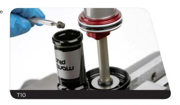
Use a T10 TORX wrench to remove the damper body bleed screw from the damper body eyelet.
