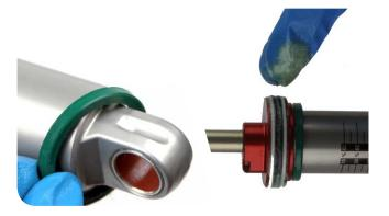
Apply a small amount of grease to the air can threads. Inject 0.5 mL of Maxima® Maxum4 Extra 15w 50 into the air can before installing the air can onto the damper. Firmly press the air can down until the sealhead/air piston is inserted into the air can
