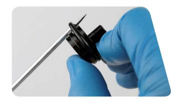
Use a 27 mm open end wrench at the base of the IFP reservoir to loosen it from the eyelet.
