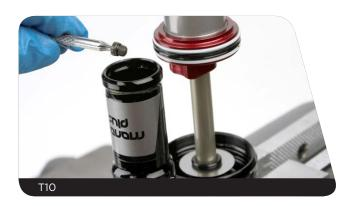
Pour additional RockShox 3wt suspension fluid into the IFP reservoir until it is level with the top of the reservoir.
