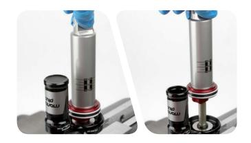
Use a T10 TORX\* wrench to install the IFP bleed screw into the IFP. The bleed screw should be submerged in fluid.
