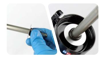
Use your fingers to remove and replace the o-ring located inside the shaft eyelet threads.
