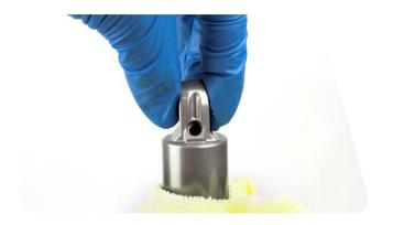
If the damper body is all the way down and air bubbles are still present, then reinstall the damper bleed screw, remove the IFP bleed screw, and repeat steps 9-12 until no more air bubbles are present.
