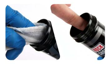
Install the first backup ring by inserting one end into the air can, then push the remainder of the ring into the can, so that it rests on the bottom of the second deepest groove.
