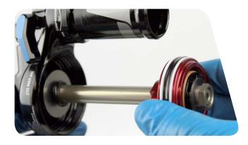
Use the RockShox Rear Shock Vise Block to clamp the damper shaft into a vise.
