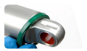
Use a 17 mm open end wrench to loosen the seal head/air piston assembly from the damper body. Use your hand to remove the assembly.
