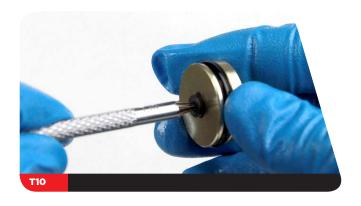
Remove and replace the IFP o-ring.
