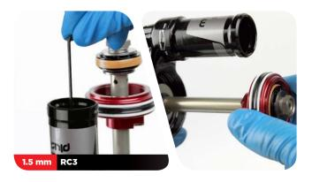
4 Use your hand to install the seal head/air piston onto the damper body.
