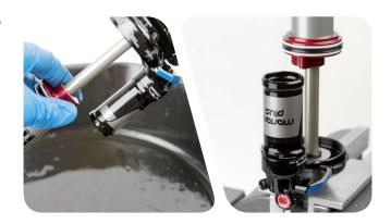
Use the Schrader valve tool to install a new Schrader valve into
