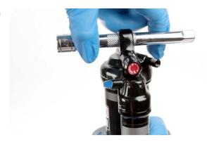
5 Stabilize the air can with a strap wrench to prevent it from rotating. Use a torque wrench with a 13 mm crowfoot socket to tighten the air can to 4.5 N m (40 in-lb).
