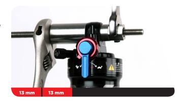
Unthread the catcher from the threaded rod. Remove the tool from the shaft eyelet and discard the old bushing.
