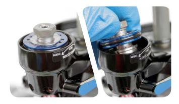
**Monarch Plus RC3 Only**: Remove and replace the compression assembly o-rings.
