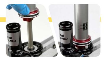
Pour RockShox 3wt suspension fluid into the IFP reservoir until it is level with the top of the reservoir.
