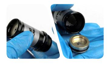
Use a T10 TORX® wrench to remove the IFP bleed screw. Replace the o-ring on the IFP bleed screw.
