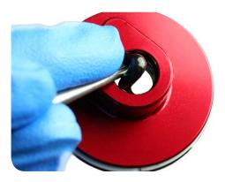
8 Use a pick to remove and replace the inner o-ring, located at the base of the threads in the seal head/air piston.
