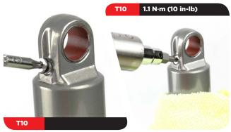
Use a T10 TORX wrench to remove the IFP bleed screw from the IFP.
