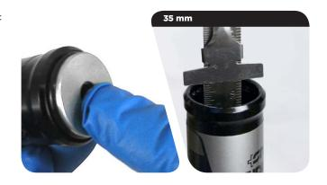
Monarch Plus™ RC3 Only: Install the compression assembly, nut side first, into the threaded side of the IFP reservoir. Push the compression assembly into the reservoir until it stops.
