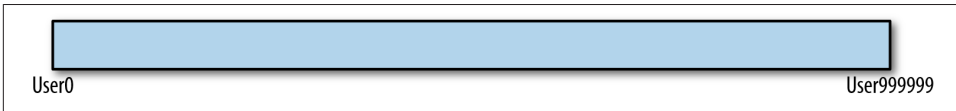
Figure 13-3. Before a collection is sharded, it can be thought of as a single chunk from the smallest value of the shard key to the largest
