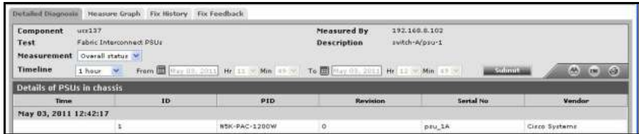
Figure 13: The detailed diagnosis of the Overall status measure of the Fabric Interconnect PSUs test
