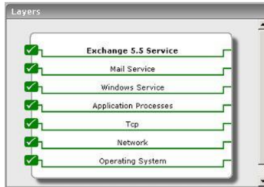
Figure 4.1: Layers of MS Exchange Server 5.5
