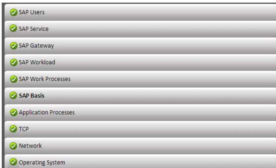
Figure 2.3: The layer model of a SAP R/3 server
