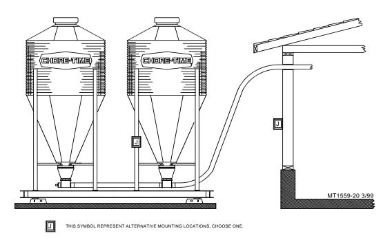
Figure 29. Mount Base Installation (side view)
