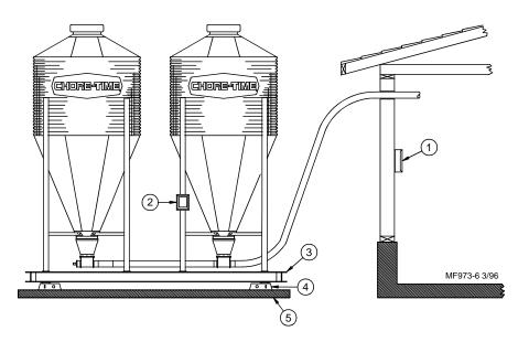
Figure 20. System components layout for (2) Bins and Bin Platform with (4) Load Cells (side view)
