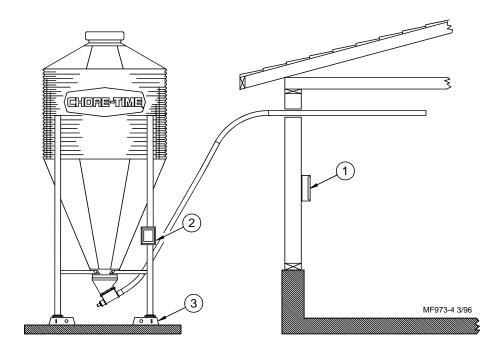
Figure 18. Components layout for 4-Legged Bin (side view)
