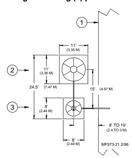
Figure 23. Bin Pad Layout and Position Diagram (top view)
