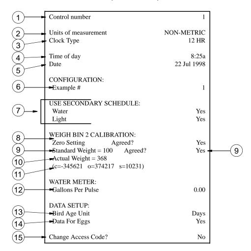
$\label{eq:continuous} \textbf{Figure 17. System Setup and Calibration default screen.}$
