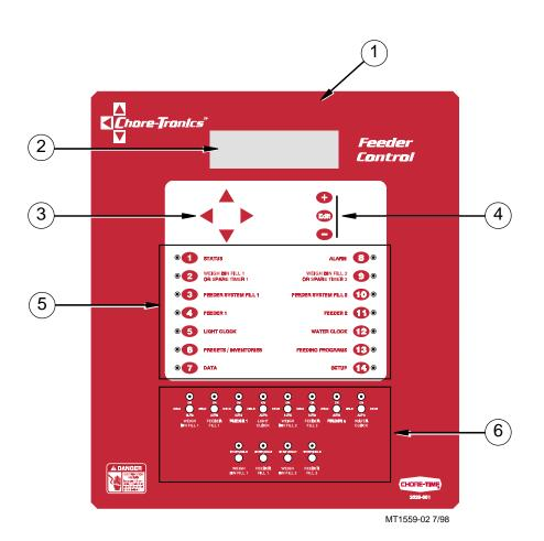
ItemDescription1Feeder Control2Viewing Screen3Navigation Buttons4Edit Buttons5Subject Buttons6Relay Switches
