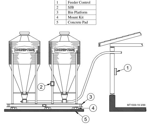
Figure 21. System components layout for (2) Bins and Bin Platform with (6) Load Cells (side view)
