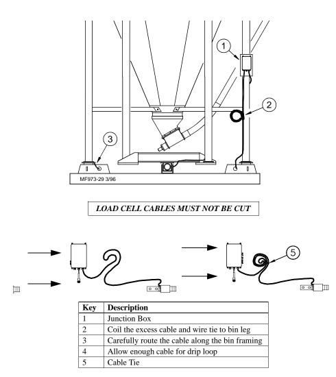
Figure 30. Cable Routing and Coiling (front view)
