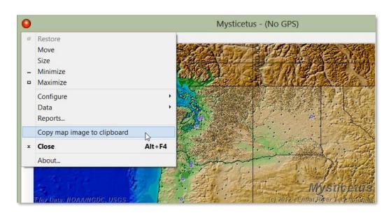
This will capture the contents of the Map Window, including all bathymetry, shapefile maps and geo-spatial objects (plans, GPS tracks, sightings, etc.) and copy it to the clipboard, where it can be pasted into any other Windows application.
