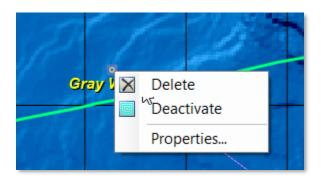
Note that some objects are marked as "Not Deletable". To see (or change) this setting, right click on the object, choose Properties... and then check the Properties window for the "Deletable" setting:
