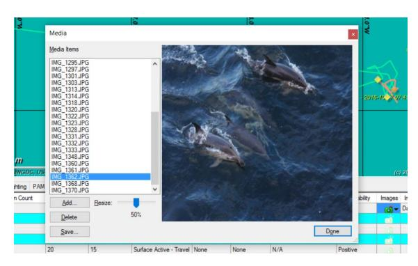
This will directly insert the selected image(s) to the sighting record and associated meta data will be tied to the photo including sighting data.
