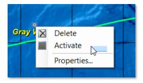
Mysticetus will draw a line from the active vehicle (vessel/aircraft) to the active waypoint and keep that updated at all times. In addition, the real-time navigation panel on the right side will be updated. Waypoints can also be activated by selecting them from the real-time navigation panel:
