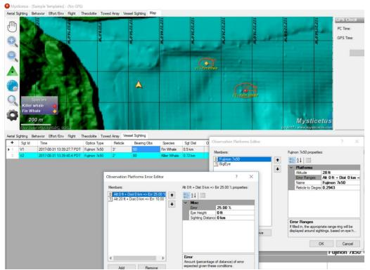
Below is an example of configuring a Fixed Error amount in Mysticetus. In this case, it's set to 100m for stations at 13m eye height and 200m for stations at 5m eye height. Mysticetus compares actual eye height at time of sighting, grabs the configured setting with the closest eye height and distance.
