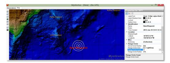
As mentioned in *section 8.3.5* - *Activation (Plans, Waypoints/Sightings)*, waypoints can then be activated and a large amount of navigation information about range, bearing, time-to-go, and so on will be displayed.
