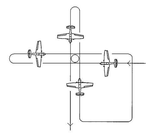
Figure 1 : Test pattern to be flown as shown. Maximum radius from test point to be 1 000 meters at any time during test
