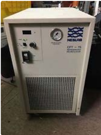
Neslab CFT-75 Circulating Chiller
