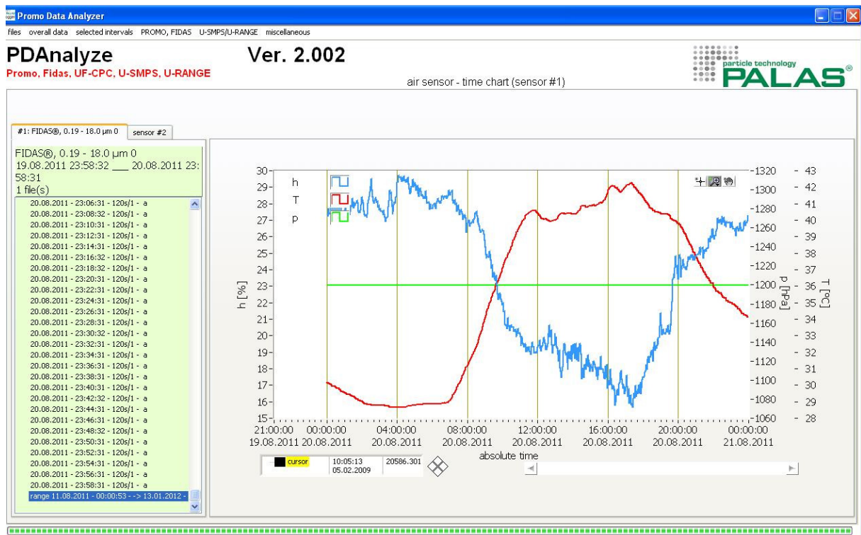
Figure 30: „ PROMO, FIDAS: air sensor - time chart “ Display of sensor data for h , T and p
