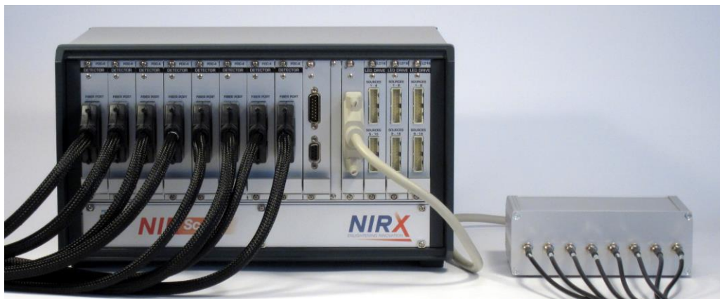
Figure 100. NIRScout devices offering laser illumination. Top: NIRScout extended Plus with integrated 2- or 4-wavelength laser illumination. Bottom: NIRScoutX with optional external 4-wavelength illumination module.
