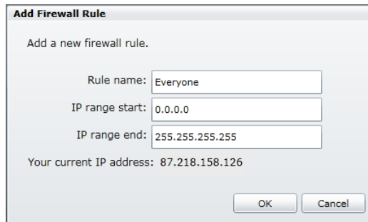
Figure 15.-Firewall rule Configuration allowing any IP
