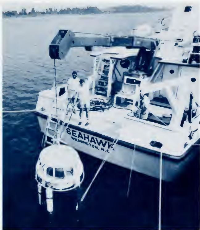
Figure 17-4 Open Bell Showing Control Lines
