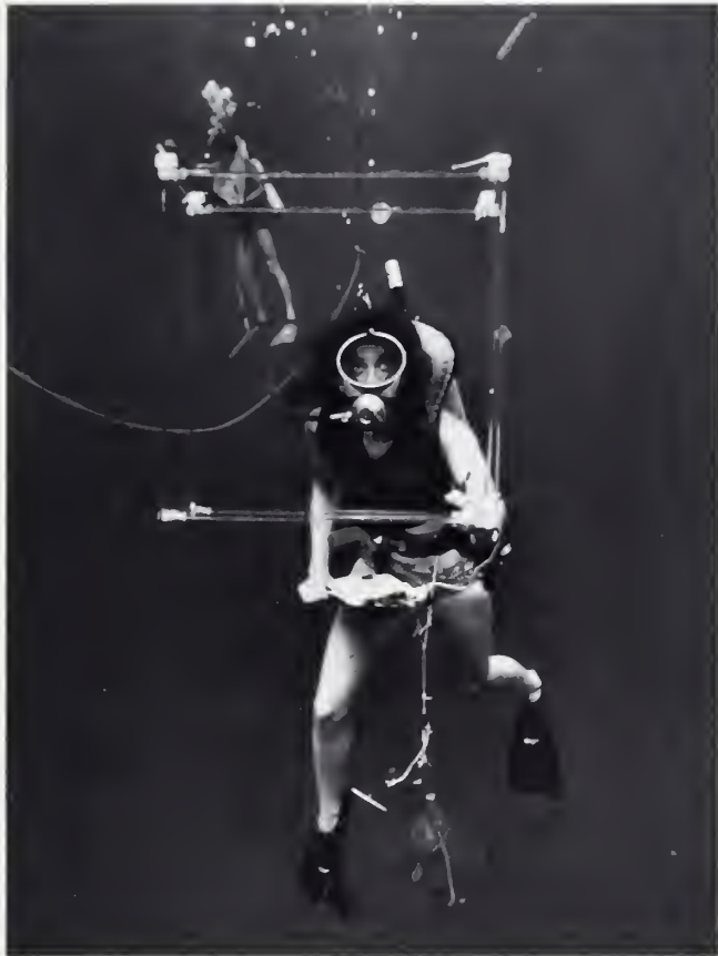
Figure 9-13 Use of a Plexiglas Reference Frame for Estimating Population Densities in Midwater
