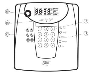
15 Buzzer - The buzzer provides an audible indication of alarm, trouble, programming and status of the system.
