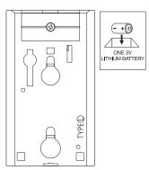
vided. Replace the sensor on its mounting plate, making sure it snaps into place. After the battery is installed, the detector will take 60 seconds to warm up. During this time the LED will flash slowly.
