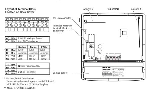
**PGM 1 and PGM 2** - are programmed in section [009], output attributes are programmed in section [141] and [142].
