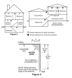
Do not locate detectors in areas of high humidity. Do not locate detectors in areas where the temperature rises above 100°F (38°C) or falls below 41°F (5°C). Smoke detectors should always be installed in accordance with NFPA 72, the National Fire Alarm Code. Smoke detectors should always be located in accordance with:
