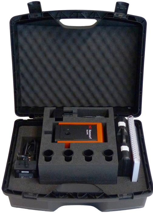
Figure 6-2: Packing. The NaioAFM system packed in its instrument case. Shown here is the NaioAFM system with optional NaioAFM Side View Camera and Isostage Adapter Set.
