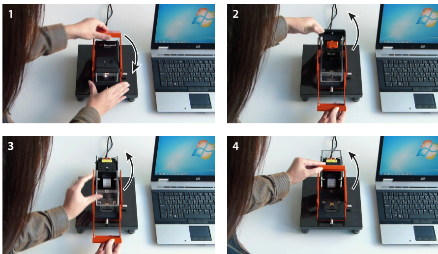
Figure 3-9: Opening the NaioAFM for full access to the sample stage. Step 1: Flip the locking handle all the way to the front. Step 2: Flip the scan head cover (and scan head) all the way to the back. Step 3: Flip the scan shield all the way to the back. Step 4: Optionally flip back the locking handle again.
