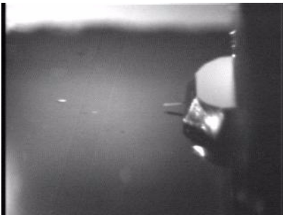
Figure 6-1: Side view of the cantilever after retracting. Minimal distance required for safe removal of the scan head and sample.
