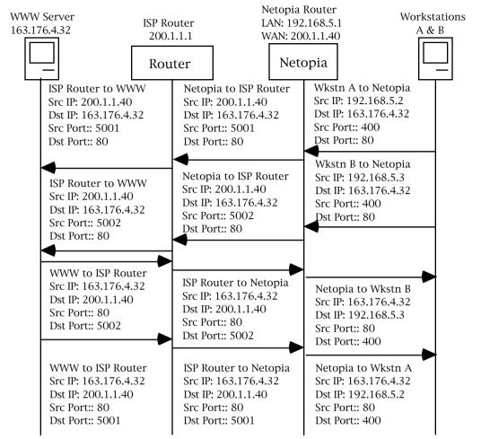
As you can see, when Workstation A and Workstation B transmit an IP packet to the WWW Server on the Internet, they have unique source IP addresses on the LAN interface but potentially the same source ports, which in this case is 400. When the Netopia R3100 receives these packets, the source IP addresses are substituted with the single globally unique IP address that was acquired on the WAN interface which is 200.1.1.40.
