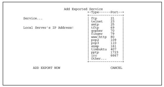
Within Exported Services is a pop-up containing a list of well known TCP and UDP services that can be redirected to a single host on the Netopia R3100's LAN interface. There is also an "Other..." option which allows for manual configuration of additional TCP or UDP ports. There can be a total of 32 Exported Services that can be defined.
