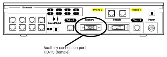
Connect the male HD-15 end of the LocalTalk cable to the **Auxiliary** port on your Netopia R3100. Connect the other end of the cable to your LocalTalk network. You can use only one connection on the Auxiliary port. You cannot use both the PhoneNET connector and an external modem.
