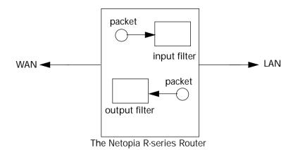
Packets in the Netopia R3100 pass through an input filter if they originate in the WAN and through an output filter if they're being sent out to the WAN.
