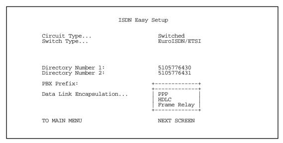
For IDSL routers, Frame Relay encapsulation is the default.
