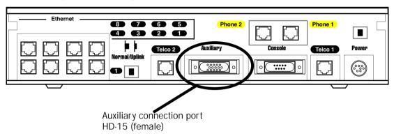
By default, the **Auxiliary** port on your Netopia R3100 is enabled for an external asynchronous modem. This means that all you have to do is connect your modem to the Auxiliary port and configure its settings in the Line Configuration screens under the WAN Configuration menu. For detailed configuration instructions see "Auxiliary Port Configuration" on page 8-10.
