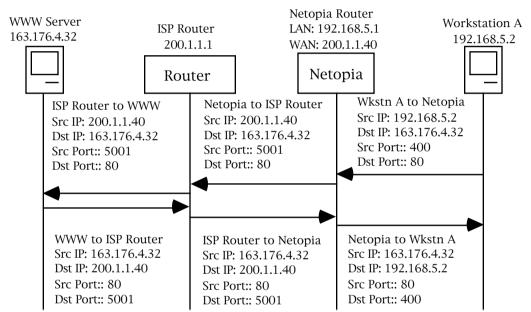
As you can see, the IP packet from Workstation A is sent to the Netopia R3100 and the source IP address is substituted with 200.1.1.40 and the source port is substituted with 5001, then the IP packet checksum is recalculated. When this modified packet reaches the WWW Server on the Internet, the WWW Server responds and sends the IP packet back to destination IP address 200.1.1.40 and destination port 5001.
