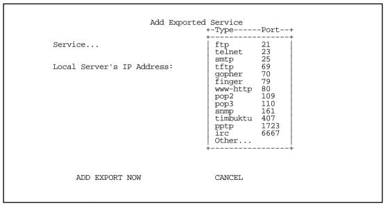
5. Select any of the services/ports and press Return to associate it with the address of a server on your local area network. For example, if we select **www-http 80**, press Return, and type **10.0.0.2**. The Netopia R3100 will then redirect any incoming traffic destined for a Web server to address 10.0.0.2.
