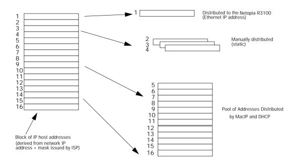
The figure above shows an example of a block of IP addresses being distributed correctly.
