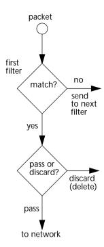
If the package does not match the first inspector's criteria, it goes to the second inspector, and so on. You can see that the order of the inspectors in the line is very important.
