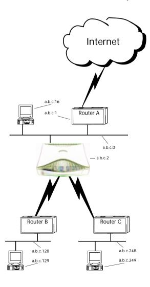
Routers B and C (which could also be Netopia R3100s) serve the two remote networks that are subnets of a.b.c.O. The subnetting is accomplished by configuring the Netopia R3100 with connection profiles for Routers B and C (see the following table).
