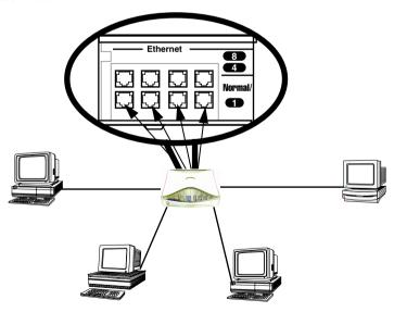
To connect your 10Base-T network to the Netopia R3100 through an Ethernet port, use a 10Base-T cable with RJ-45 connectors.
