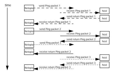
**Packets Lost:** The number of packets unaccounted for, shown in total and as a percentage of total packets sent. This statistic may be updated during the Ping test, and may not be accurate until after the test is over. However, if an escalating one-to-one correspondence is seen between **Packets Out** and **Packets Lost**, and **Packets In** is noticeably lagging behind **Packets Out**, the destination is probably unreachable. In this case, use **STOP PING**.
