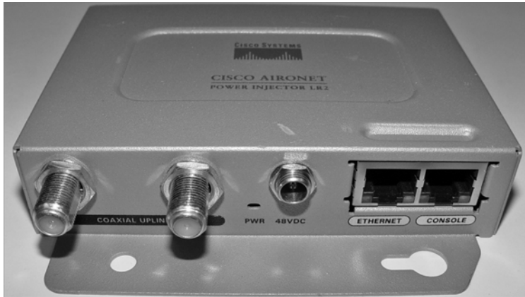
FIGURE 11.23 Wireless bridge power injector
