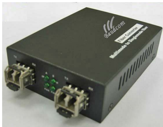
FIGURE 3.15 Single-mode to multimode fiber
