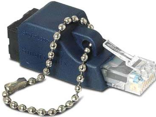
FIGURE 18.16 Ethernet loopback plug
