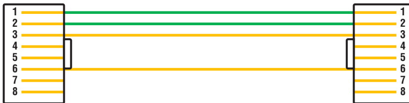
FIGURE 3.21 Straight-through Ethernet cable
