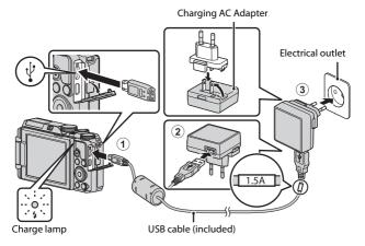
If a plug adapter\* is included with your camera, securely connect it to the Charging AC Adapter. Once the two are connected, attempting to forcibly remove the plug adapter could damage the product.
