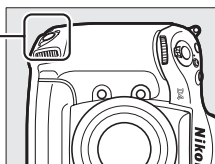
Vertical shooting shutter-release button lock
