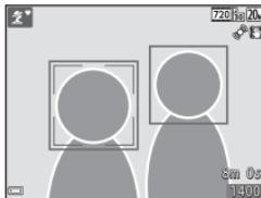
When the camera detects more than one face, the double border (focus area) is displayed around the face that is focused on, and single borders around the others.
