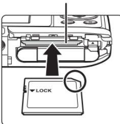
Be Careful to Insert the Memory Card in Correct Direction
