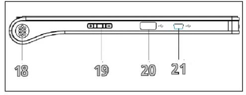
*18. Left Speaker:* This is the left side speaker. The audio from the device is outputed through speakers while there is no audio jack plugged in.
