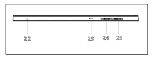
*22. Microphone:* This is the microphone, which can be used for audio input while using apps like Viceo Recorder and other voice chat features.
