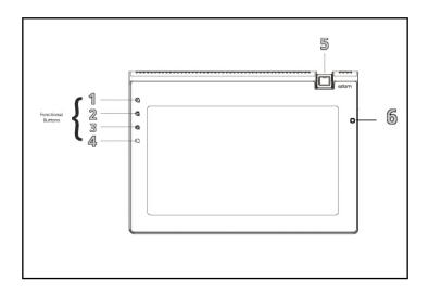
*1. Search:* On Single Tap, the Search feature is enabled for the app, if there is any. Logn pressing the the search button will controls the Back lit LCD. If the device has a transreflective screen, switching off the back lit LCD screen will enable the PixelQi screen. If the device has a normal LCD screen, switching off the LCD will turn the display off.
