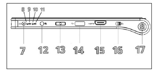
*7. Power Port:* This port is for the Adapter to be plugged in to charge the device.
