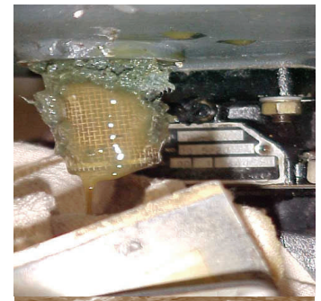
The oil sump screen was clogged with a shop towel.
