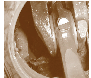
Post Accident Engine Tear-down Reveals Paper Shop Towel in The Crankcase
