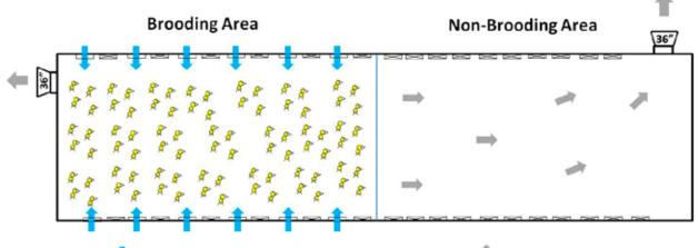
💠 = Air Inlet Opened 🛛 📼 = Air Inlet Closed 🛛 👕 = Exhaust Air
