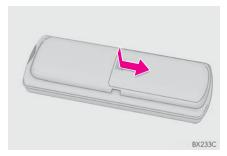
2 Remove the depleted batteries and install new batteries.
