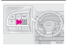
The voice command system and its list of commands can be operated. (→P. 250)
