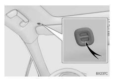
• It is unnecessary to speak directly into the microphone when giving a command.
