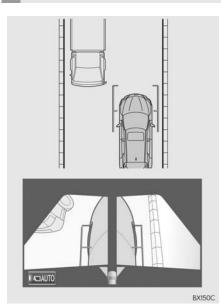
Check the positions and distance between the vehicle width guide line and a target object such as the obstacle or curb of the road.
