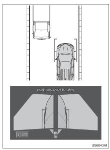
Check the positions and distance between the vehicle width guide line and a target object such as the obstacle or curb of the road.
