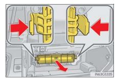
The "TUP" marks shown on the filter and the filter case should be pointing up.
