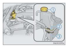
If the level is on or below the "LOW" line, add coolant up to the "FULL" line.  $(\to\!P\!.\,509)$
