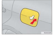
2 Turn the fuel tank cap slowly to remove it and put it into the holder on the fuel filler door.
