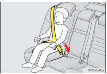
Check that the shoulder belt is correctly positioned over the child's shoulder and that the lap belt is as low as possible.  $(\rightarrow P.36)$
