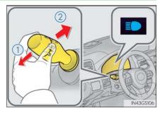
AFS (Adaptive Front-lighting System) secures excellent visibility at intersections and on curves by automatically adjusting the direction of the light axis of the headlights according to vehicle speed and the degree of the tire's angle as controlled by steering input.
