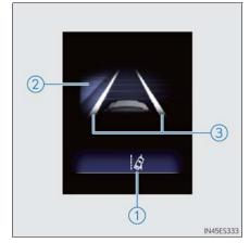
Indicates that steering wheel assistance of the steering assist function or lane centering function is operating.
