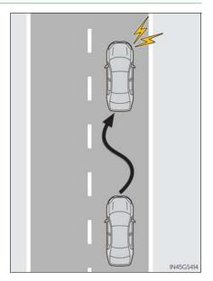
This function is linked with radar cruise control and provides the required assistance by operating the steering wheel to keep the vehicle in its current lane.
