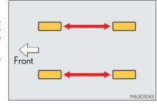
► Vehicles with front and rear tires of differing sizes Tires cannot be rotated.
