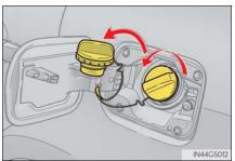
■ When the fuel filler door cannot be opened by pressing the rearward of the fuel filler door
