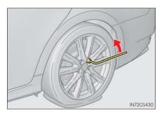
Turn the tire jack portion "A" by hand until the notch of the jack is in contact with the jack point.
