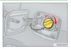
2 Close the fuel filler door, and press the center of the rear edge of the fuel filler door until you hear a click. When you lock the doors, the fuel filler door will lock also.
