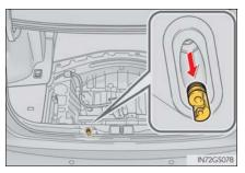
4 Insert the tool and press it down firmly while turning it counterclockwise until it stops.
