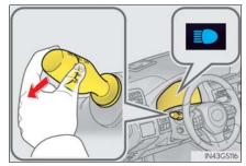
2 Press the Automatic High Beam switch.
