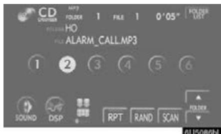
While the disc is playing, touch “SCAN” on the screen and hold it until the “FLD-SCAN” appears on the screen.
