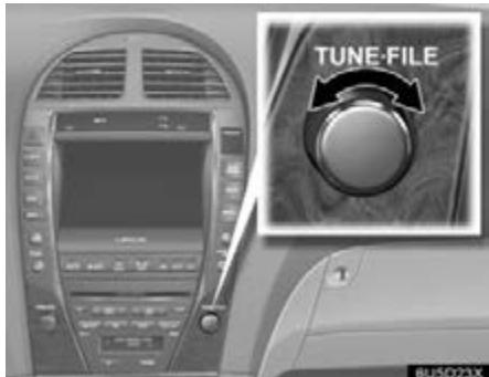
**Turn the knob clockwise to step up the station band or counterclockwise to step down.**
