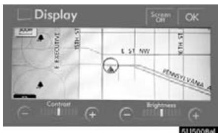
1. Touch the desired button to adjust contrast and brightness.
