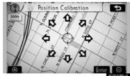
2. Touch the eight directional touch-screen button to move the cursor
