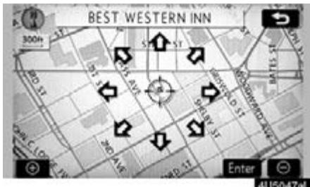
2. Touch the eight directional touch-screen button to move the cursor
