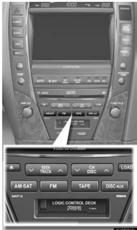
Push “AM-SAT”, “FM”, “TAPE” or “DISC-AUX” button to turn on the desired mode. The selected mode turns on immediately.
