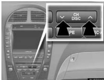
1. Push the “ $\wedge$ ” or “ $\vee$ ” button of “CH/DISC” or touch the disc number button on the screen to highlight the disc number you want to eject.
