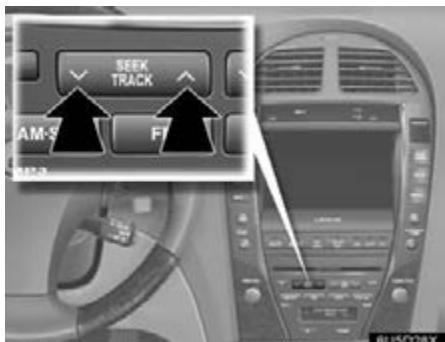
**“SEEK/TRACK” button:** Use for a direct access to a desired track.
