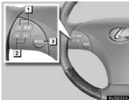
Some parts of the audio/video system can be adjusted with the switches on the steering wheel.
