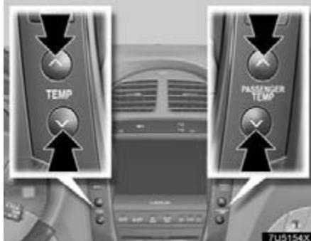
2. Use the "TEMP" or "PASSENGER TEMP" button to set the desired vehicle interior temperature.
