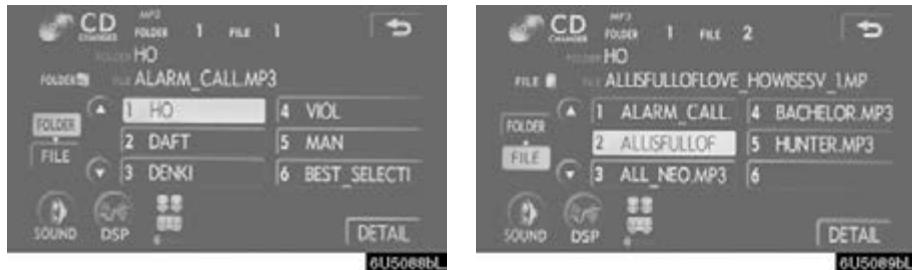
**“FILE”:** The desired file can be selected in a list. This function is available only when the vehicle is not moving.
