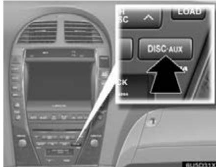
Push the “DISC-AUX” button if the disc are already loaded in the CD changer.
