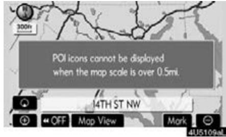
This message appears when the system is in the POI mode and the map scale is over 0.5 miles (800 m).
