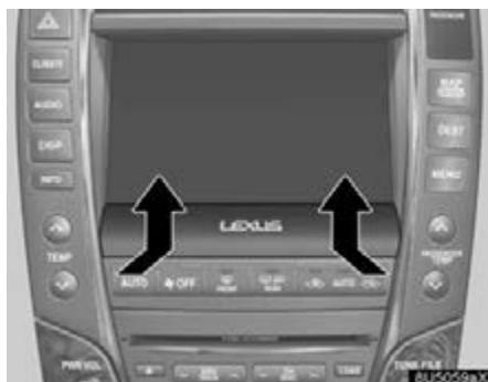
2. Push the cover, and slide it upward to remove it.
