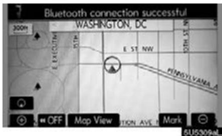
When the “ENGINE START STOP” switch is in the ACCESSORY or IGNITION ON mode and the Bluetooth® is automatically connected, the connection check is displayed.
