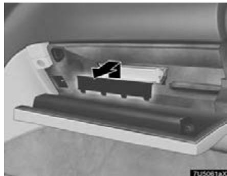
2. Open the glove box. Remove the glove box cover.
