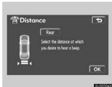
Touch “Rear” to switch the distance for the back sensors display and tone indication, from long distance to short distance, or from short distance to long distance.
