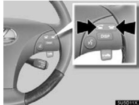
By pushing the telephone switch above, you can receive a call or hang up without taking your hands off the steering wheel.
