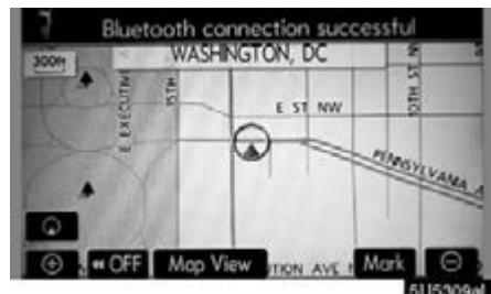
When the "ENGINE START STOP" switch is in ACCESSORY or IGNITION ON mode, the selected Bluetooth® phone will be automatically connected and the connection result is displayed.
