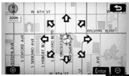
When an arrow facing the desired point is touched, the map scrolls in that direction. Releasing the finger from the arrow will stop the scrolling.
