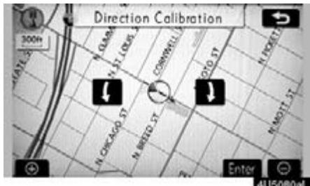
4. Touch either or to adjust the direction of the current vehicle position mark.
