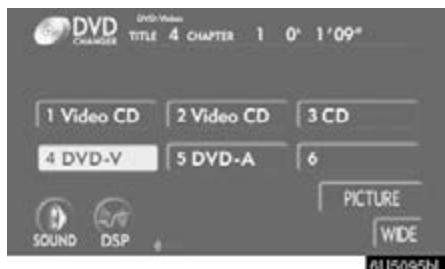
Push the "AUDIO" button to display this screen. You can operate the touch-screen buttons and choose the number of the disc you want to play. The selected disc is automatically played.
