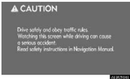
After about 5 seconds, the "CAUTION" screen automatically switches to the map screen. When the "MAP/VOICE" button is also pushed, the map screen is displayed.
