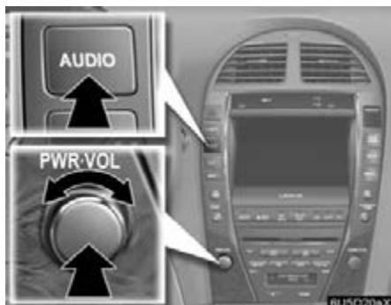
**“PWR-VOL”:** Push this knob to turn the audio system on and off. Turn this knob to adjust the volume. The system turns on in the last mode used.
