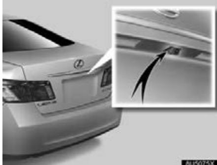
The rear view monitor system camera is located on the trunk as shown in the illustration. The camera uses a special lens. The distance of the image that appears on the screen differs from the actual distance.
