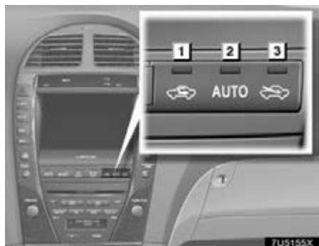
Each time you push the air intake control button, the mode changes in order from the RECIRCULATED AIR mode to AUTOMATIC mode to OUTSIDE AIR mode, then back to the RECIRCULATED AIR mode. Each indicator light shows which mode is now selected.
