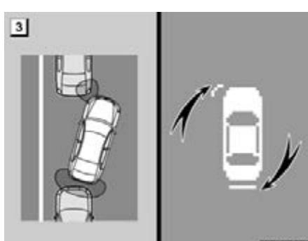
When obstacles are detected on the front and rear of the vehicle at the same time; the multi-information display and screen illuminate their relevant indicator bars. And beeps are as follows:
