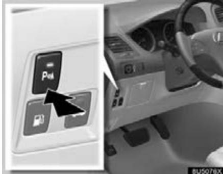
The Intuitive parking assist is a warning system used when parking the vehicle at low speed (e.g. into a garage). It uses an ultrasonic sensor, which checks the approximate distance to an obstacle. It will inform you of the approximate distance to an obstacle by displaying information on the multi-information display and the screen, and with beeping sounds.
