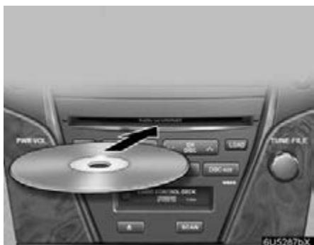
2. Insert only one disc while the CD changer door is open.
