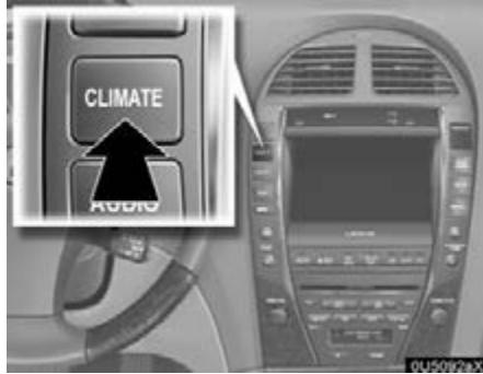
**"CLIMATE":** Push this button to display touch-screen buttons for automatic air conditioning controls.
