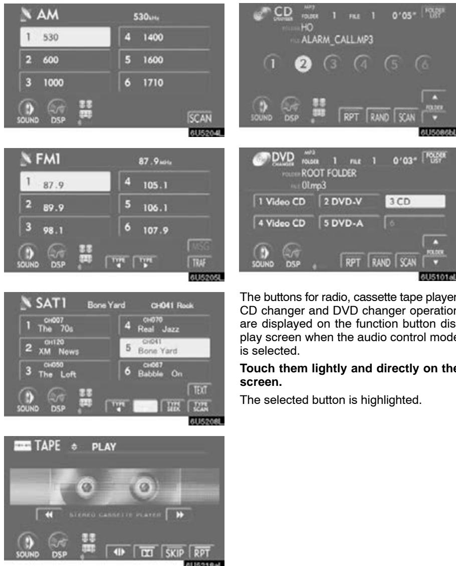
The buttons for radio, cassette tape player, CD changer and DVD changer operation are displayed on the function button display screen when the audio control mode is selected.
