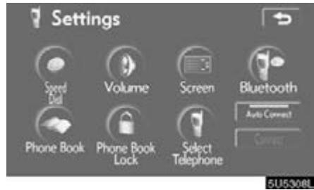
When you register your phone, auto connection will be turned on. Always set it to this mode and leave the Bluetooth® phone in a condition where connection can be established.
