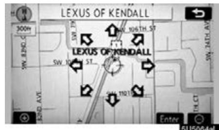
2. Touch the eight directional touch-screen button to move the cursor
