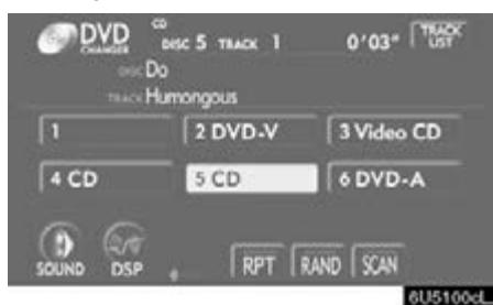
The numbers of the trays where the disc is not set are dimmed.
