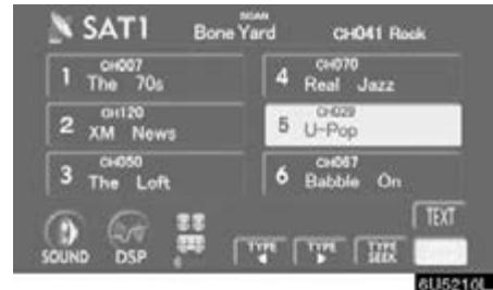
**To scan the currently selected channel category:** Touch “**TYPE SCAN**” or push the “**SCAN**” button briefly. “**SCAN**” appears on the display. The radio will find the next channel in the same channel category, stay there for a few seconds, and then scan again. To select a channel, touch “**TYPE SCAN**” or push the “**SCAN**” button a second time.
