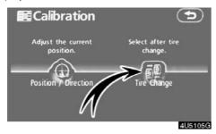
To perform a distance calibration procedure, touch "Tire Change" on the "Calibration" screen.
