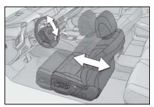
On vehicles with adjustable seat cushion side bolsters, when the driver's door is opened with the power switch off, the seat cushion side bolsters will lower if they are in the default position.
