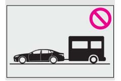
Your vehicle is not designed to be dinghy towed (with 4 wheels on the ground) behind a motor home.
