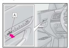
Using the seat adjustment switches on the driver's seat, adjust the front passenger's seat.
