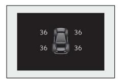
If the tire pressure drops below a predetermined level, the driver is warned by a screen display and a warning light. (→P.431)
