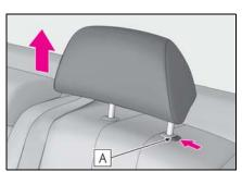
Removing the head restraints (power head restraints)
