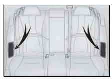
There are air intake vents on each side of the rear seatback with the purpose of cooling the hybrid battery (traction battery). If the vents become blocked, hybrid battery output may be reduced.
