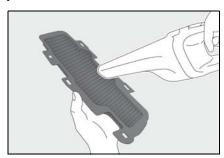
Install the filter in its original position, and then install the grille.
