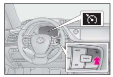
Accelerate or decelerate, with accelerator pedal operation, to the desired vehicle speed (at or above approximately 25 mph [40 km/h]) and press the "-SET" switch to set the speed.
