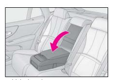
▶ Vehicle with power rear seat Pull the lock release lever and fold the rear seatback down.
