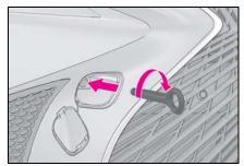
4 Tighten down the towing eyelet securely using a phillips-head screwdriver or hard metal bar.
