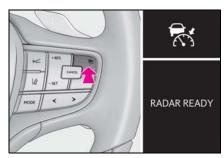
Accelerate or decelerate, with accelerator pedal operation, to the desired vehicle speed (at or above approximately 30 mph [50 km/h]) and press the "-SET" switch to set the speed.
