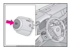
2 Push the lever away from you with the headlight switch in the D or AUTO position.
