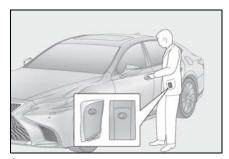
2 Open the hood. Remove the driver side engine compartment cover
