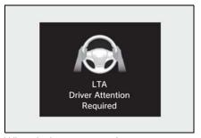
When the lane centering function is operating and the system determines that the vehicle may depart from its lane due to a sharp curve, etc., a warning display urging the driver to operate the steering wheel, will be displayed.
