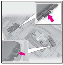
3 Remove the fuse with the pullout tool.
