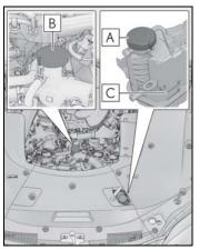
Add coolant through the inlet of the cap
