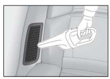
If "Maintenance Required for Traction Battery Cooling Parts See Owner's Manual" is displayed on the multi-information display, the filters may be clogged. Remove the air intake vent grilles and clean the filters.
