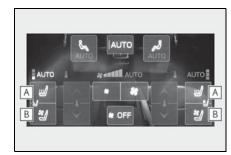
Adjust the rear seat heater temperature level
