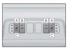
A Increases the rear seat heater temperature level
