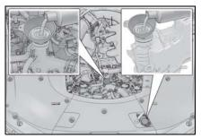
Start the hybrid system and turn the air conditioning system on to check that the radiator cooling fan operates and to check for coolant leaks from the radiator or hoses.
