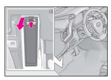
► Passenger's side instrument panel Push the tab in and remove the lid. Make sure to push the tab in during removal or installation.
