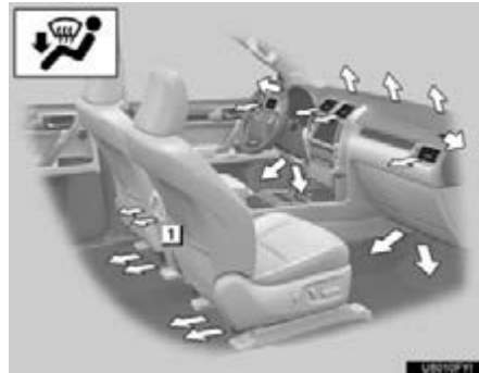
► Air flows to the feet and the windshield defogger operates (Floor/windshield)
