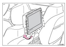
● The display angle can be adjusted between 0 degree to 50 degree.
