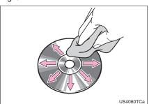
**To clean a disc:** Wipe it with a soft, lint-free cloth that has been dampened with water. Wipe in a straight line from the center to the edge of the disc (not in circles). Dry it with another soft, lint-free cloth. Do not use a conventional record cleaner or anti-static device.
