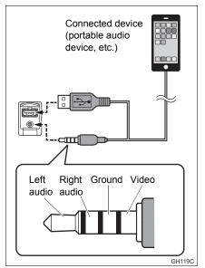
When using an iPod video, a cable that has a 4-pole AUX plug and a USB connector is necessary. Connect the plug and connector to the AUX and USB ports.
