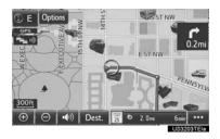
When the vehicle is receiving signals from satellites, the "GPS" mark appears at the top left of the screen.
