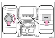
"PWR·VOL" knob: Press to turn the audio/visual system on and off. The system turns on in the last mode used. Turn this knob to adjust the volume.
