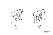
Insert a new fuse of the same amperage rating, and make sure it fits tightly. If it does not fit tightly, have an expert install it. We recommend your Toyota dealer.
