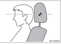
To raise a head restraint, pull it up to the desired position.
