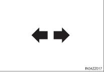
If an indicator light stays on without flashing or if it flashes abnormally, one of the turn signal bulbs may be burned out.
