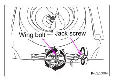
If the jack is not completely secured, it could rattle while driving. Make sure the jack screw is sufficiently tightened.
