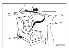
Push the child-restraint system firmly into the vehicle seat. Be sure the belt retracts as snugly as possible. A clicking noise from the retractor will be heard during retraction if the system is in the automatic locking mode. If the belt does not lock the seat down tight, repeat this step.
