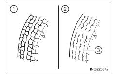
Tires degrade over time, even when they are not being used on the road. It is recommended that tires generally be replaced when they are 6 years or older. Heat caused by hot climates or frequent high loading conditions can accelerate the aging process. You should replace the spare tire when you replace the other road tires due to the aging of the spare tire. The period in which the tire was manufactured (both week and year) is indicated by a 4-digit number.
