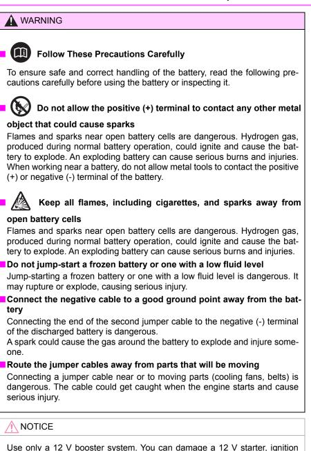
Use only a 12 V booster system. You can damage a 12 V starter, ignition system, and other electrical parts beyond repair with a 24 V power supply (two 12 V batteries in series or a 24 V motor generator set).
