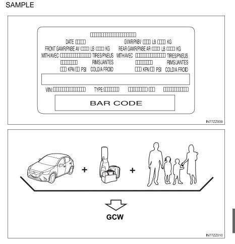
GCW (Gross Combination Weight) is the weight of the loaded vehicle (GVW).
