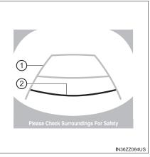
The red and yellow lines indicate the points about 19 in. (500 mm) for the red line and 39.3 in. (1000 mm) for the yellow lines from the rear bumper (at the center point of each of the lines).
