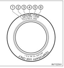
T115/70D16 90M is an example of a tire size and load index rating. Here is an explanation of the various components of that tire size and load index rating. Note that the tire size and load index rating may be different from the example.
