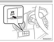
Press the switch again to turn the TCS/DSC back on. The DSC OFF indicator light will turn off.
