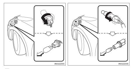
6 Install the new bulb in the reverse order of the removal procedure.
