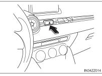
Depress the hazard warning flasher and all the turn signals will flash. The hazard warning indicator lights in the combination meter flash simultaneously.
