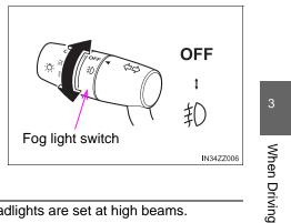
The fog lights will turn off when the headlights are set at high beams.
