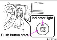
7 Press the push button start after both the KEY indicator light (green) in the combination meter and the push button start indicator light (green) illuminate.
