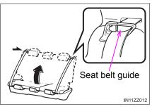
2 Press the seatback rearward and lock it in place. After returning the seatback to its upright position, make sure it is securely locked.
