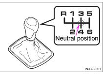
Your vehicle is equipped with a device to prevent shifting to R (reverse) by mistake. Push the shift lever downward and shift to R.
