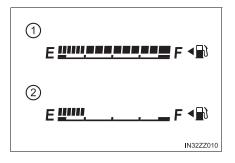
If the low fuel warning light illuminates or the fuel level is very low, refuel as soon as possible.
