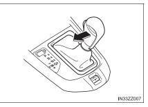
To return to automatic shift mode, shift the lever from M to D.
