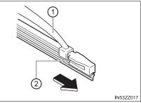
3 Remove the metal stiffeners from each blade rubber and install them in the new blade.
