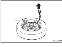
13Pass the belt through the<br/>buckle, then pull the belt end to<br/>secure the flat tire.
