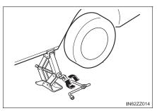
9 Remove the lug nuts by turning them counterclockwise; then remove the wheel and center cap.
