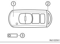
To use the auxiliary key, press the knob and pull out the auxiliary key from the smart key.
