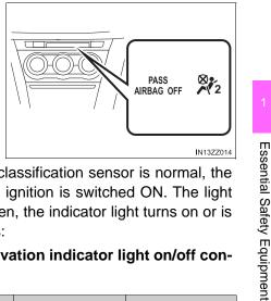
If the front passenger occupant classification sensor is normal, the indicator light turns on when the ignition is switched ON. The light turns off after a few seconds. Then, the indicator light turns on or is off under the following conditions:
