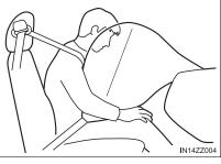
In addition, the front passenger air bag is designed to only deploy in accordance with the total seated weight on the front passenger seat. For details, refer to the front passenger occupant classification system ( $\rightarrow$ P. 78).
